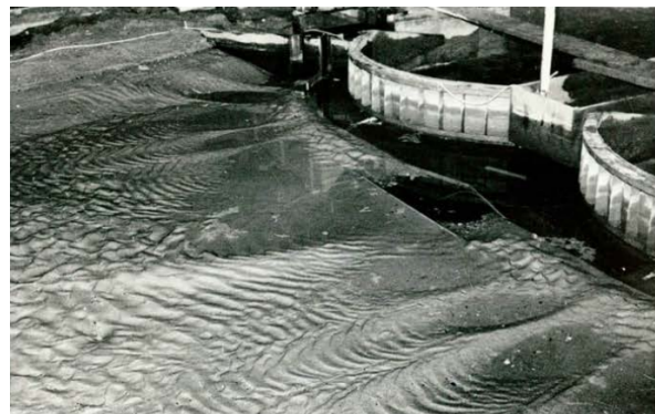
Figure 1.2: Bed damage of scale model of weir Hagestein (Waterloopkunding Laboratorium, 1955 )
