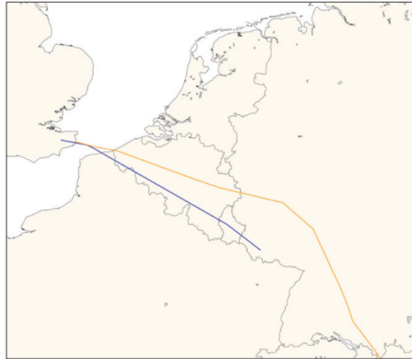
Figure 2.8: A situation where the flown trajectory (blue) is different from the planned trajectory (yellow), from [33]. In this scenario, a Belgian military airspace opened for commercial flights which allows the short-cut to be performed.
