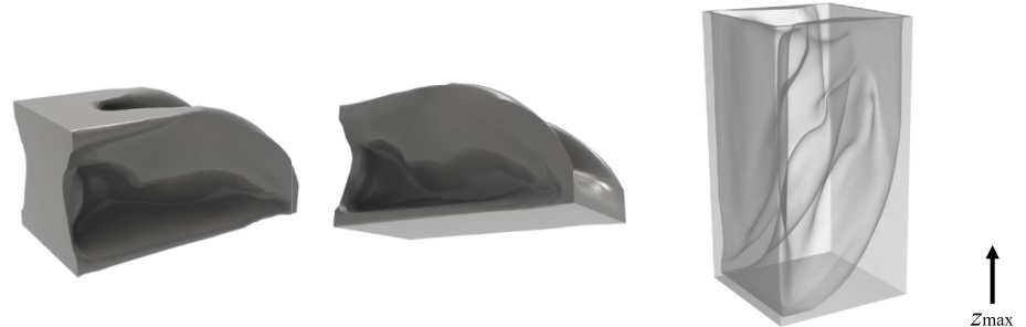
(d) Optimized beam with formwork printing direction of z_{\max}
