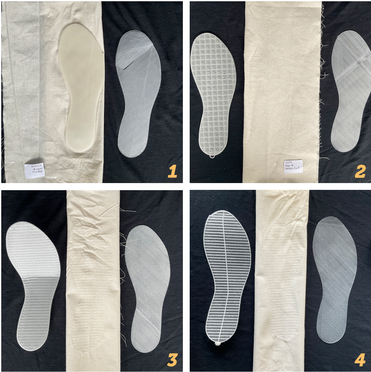
Figure 39. The “EoL” separation test setup led to adhesive failure for all the designs. For design 1 (image 1), one-sided adhesive separation occurred at the layers below the textile (bottom layer type). Designs 2 (image 2), 3 (image 3) and 4 (image 4) resulted into material separation due to two-sided adhesive failure. During separation, polymer cohesive failure occurred for designs 1 and 3.
