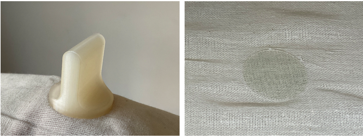
Figure 20: The dolly used, size: 23.8 x 24 mm (Malengier et al., 2018; Gorlachova & Mahltig, 2021). Top side (left) and bottom side (right).
