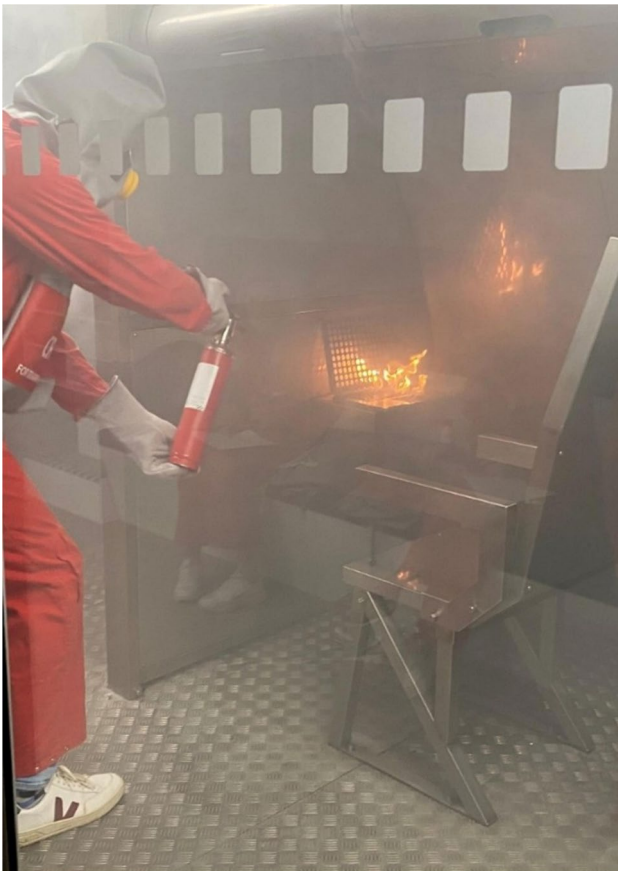
Fig. 3 The interior of the Flame Aviation fire training device. This picture shows a laptop fire scenario
