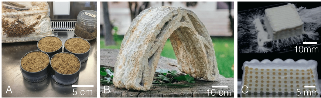
Figure 6: A: The conventional manufacturing method of MBC using moulding of inoculated substrate material [78]. B: 3D printing of substrate containing pastes allows more design freedom in MBC structures [75]. C: 3D printing of mycelium-laden hydrogels allows the manufacturing of structures with controlled nutrient supply and mycelium microstructures [1].
