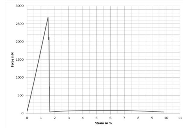
**Figure 3: Linear, fiber dominated behaviour of 0°-ePreg layer**
