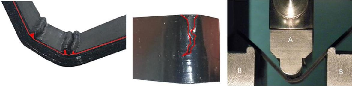
**Figure 6: Failure of 3-PT-Bending specimen (single ply delamination (l.), tensile failure (c.)) and the test set-up (r.)**
