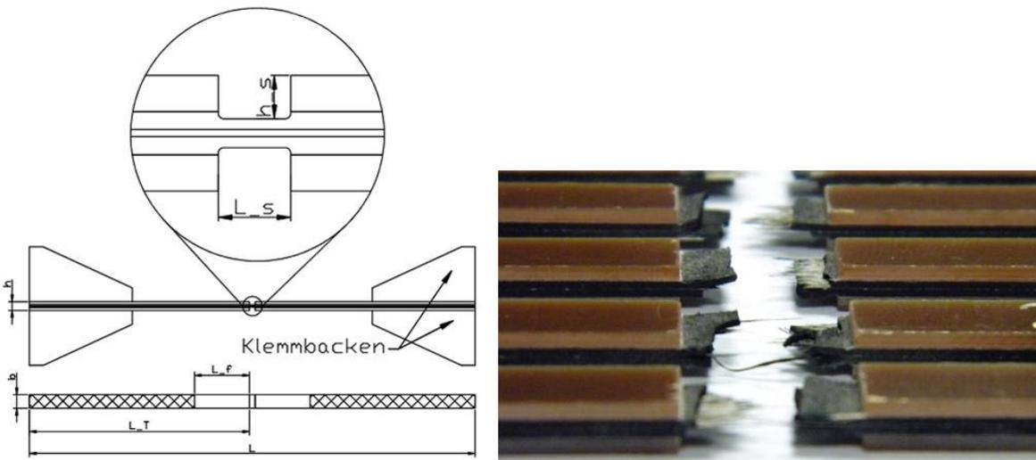
**Figure 7: Geometry of Fiber-Bundle-Pull-Out specimen (l.) and the failure (r.)**
