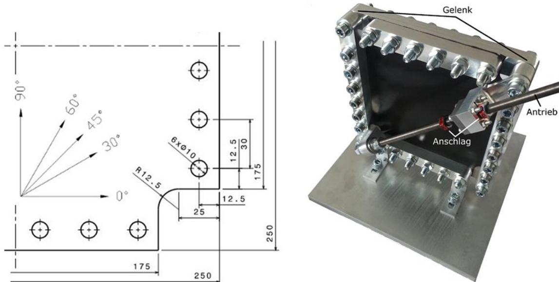
**Figure 8: Elastic skin specimen geometry (l.) and shear frame (r.) for the evaluation of elastic skin behaviour under shear load**
