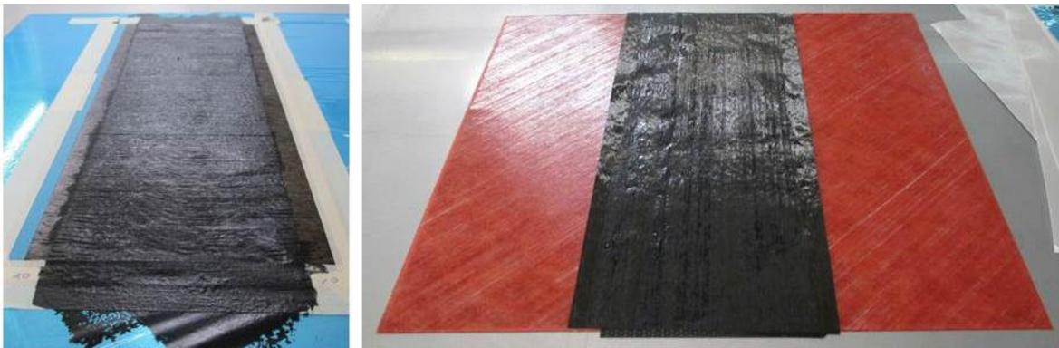
**Figure 1: Manufacturing and integration of ePreg tensile specimen**
