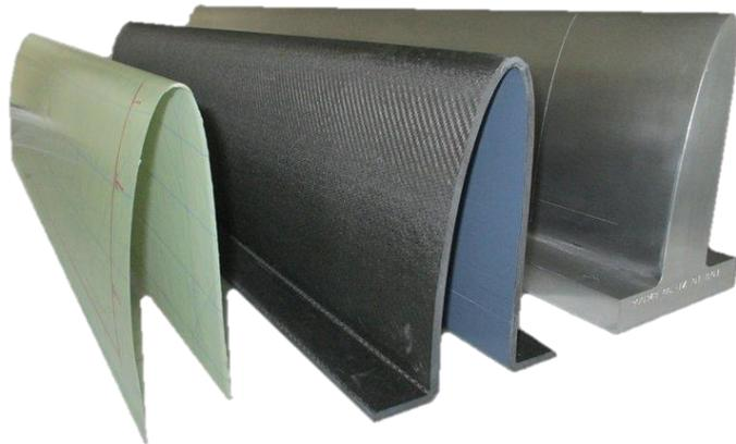
**Figure 14: 1st prototype part of the TUD-LE (l.); composite female mold (c.); aluminium mastermold for the morphing LE-elements in CHANGE (r.)**
