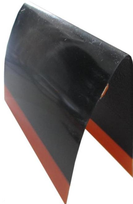
**Figure 12: The DLR-LE with a rigid ends for the clamping to the aux spar, a foam core omega stringer and a combination of a epoxy prepreg structure and elastomeric cover layers**
