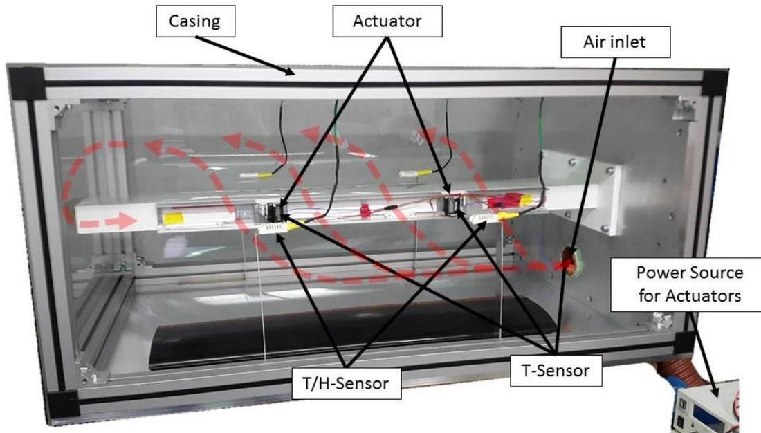
**Figure 18: The test stand box for the skin testing at elevated temperatures, high humidity and UV radiation. The set up includes several sensors for actuator temperature, temperature at the air inlet and humidity/temperature in the box. In the rear of the wing box the TUD-TE is fully integrated for the testing (Not shown are the UV radiator and the heater system).**
