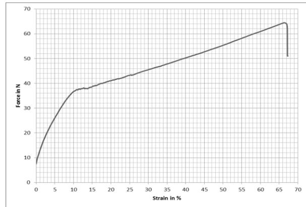
**Figure 2: Non-linear, matrix dominated behaviour of 90°-ePreg layer**
