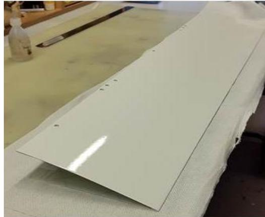
**Figure 16: Flush fit of the TUD-TE slot plate and the integrated doubler on the upper shell of the TE (top) and the TUD-TE-Element ready for delivery to TEK where mounting to the wind tunnel test wing was done (bottom)**
