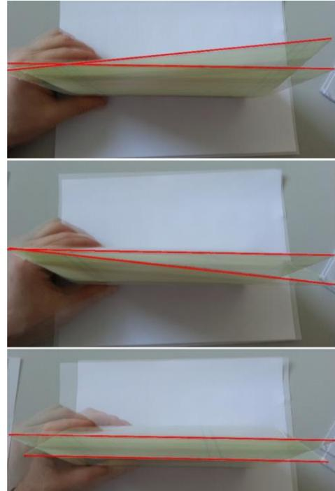
**Figure 11: Overlaid positions of possible morphing for the TUD-TE concept using conventional epoxy prepreps**
