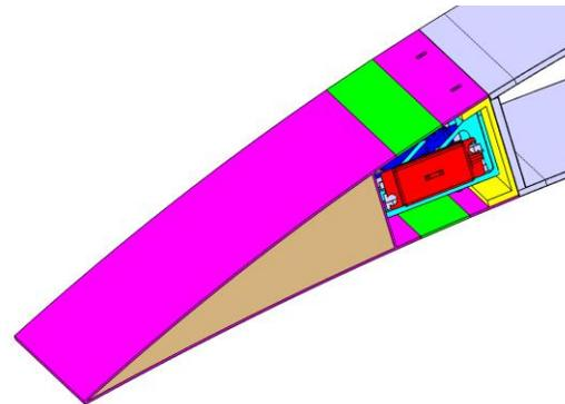
**Figure 10: The CAD-model of the original METU-TE design using two compliant skin areas (green) and five actuators**
