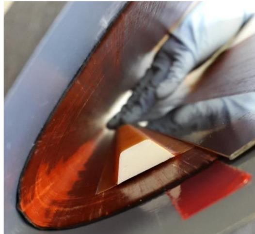
**Figure 17: Placing the premanufactured solid foam core stringer in the very limited space of the DLR-LE**
