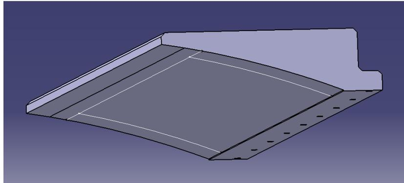
**Figure 13: Tooling for the casting of the upper surface of the NACA6510 trailing edge. The white lines indicate projected engravings on the mould surface to allow accurate post processing.**
