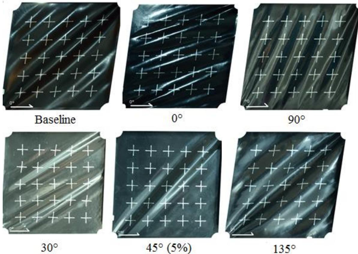
**Figure 9: A choice of skin specimen with different fiber orientations at 10% diagonal strain**
