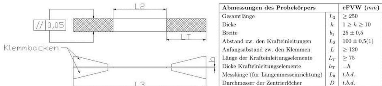
**Figure 4: Proposed and applied dimensions for the tensile testing of ePreg specimen**
