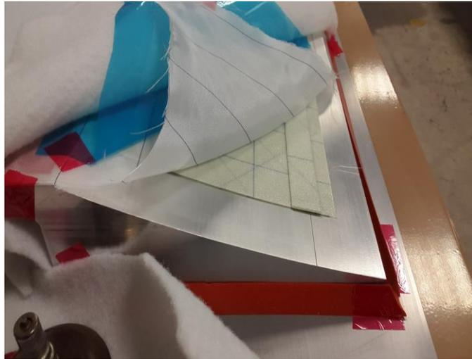
**Figure 15: The upper shell of the TUD-TE before the sealing for the autoclave cycle**
