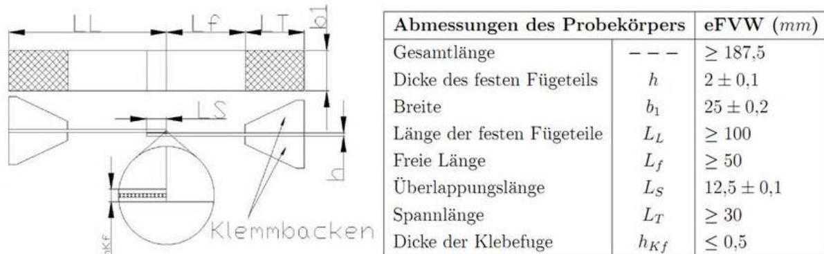
**Figure 5: Proposed and applied dimensions for the single lap shear testing of ePreg specimen**
