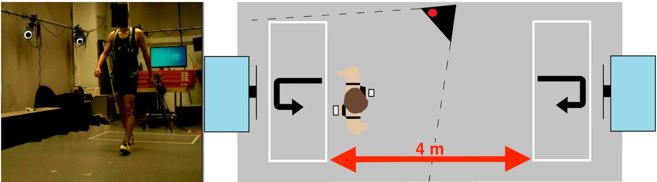
Figure 6: *Left*: Participant in the motion capture lab wearing experimental clothing, a safety harness and reflective markers. *Right*: An illustration of the experimental set-up. The triangle represents the camera that captured the image on the left. Monitors capable of displaying the biofeedback were placed at each end of the 6 meter walkway. The white boxes with the arrow are the turning areas. The distance between the turning areas is 4 meters.
