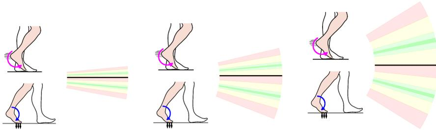
Figure 9: Three examples of the colour-shaded areas for three different reference signals. The natural ankle angles for push-off and toe clearance in the figure are respectively: *Left*:  $5^\circ$  plantarflexion  $2^\circ$  dorsiflexion, *Middle*:  $10^\circ$  plantarflexion  $5^\circ$  dorsiflexion, *Right*:  $15^\circ$  plantarflexion  $12^\circ$  dorsiflexion
