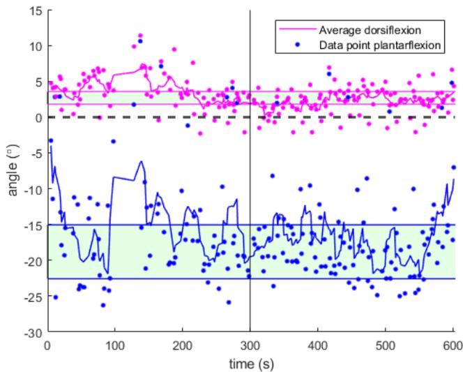
Figure 9: The feedback parameters’ angles used during a participant’s second feedback trial. The dorsiflexion angles and reference are in magenta. The plantarflexion angle and reference are in blue. The individual data points are shown as well as a moving average of six data points. The vertical black line indicates the time during the trial when the biofeedback was switched off.
