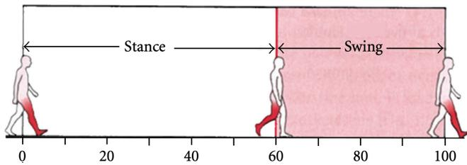
Figure 1: *Adapted from [6].* Simple representation of the gait cycle. The right leg (red) is the limb of interest. The stance period (white) is the first 60% of the cycle. The swing period (pink) is the remaining 40% of the cycle. Push-off occurs at 60% and toe clearance occurs at 80%. The active range of motion of the ankle is defined as the difference between the maximum plantarflexion and dorsiflexion angles during the swing period.
