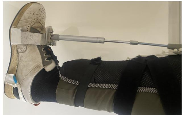
Figure 5: Impeding shoe which decreases active ankle range of motion by applying a force (80N) to the shin and foot when retracted and by damping ( $7 * 10^2$  Ns/m). The shin guard and embedded frame ensured that no excessive pressure was applied. The shoes and gas spring rod were interchangeable to ensure a personalised fit for each participant.
