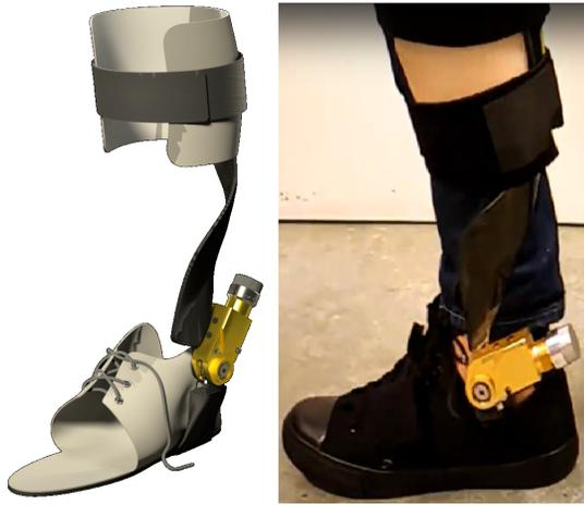
Figure 2: Adapted from [20]. *Left:* Negative-stiffness ankle-foot orthosis designed to compensate for increased joint stiffness in stroke patients with spastic paresis of the leg. The spring-loaded hinge with adjustable cam (yellow) connects the foot and brace sections (black). The in-shoe and calf cuff (beige) ensure user comfort. *Right:* Image of the orthosis in use.
