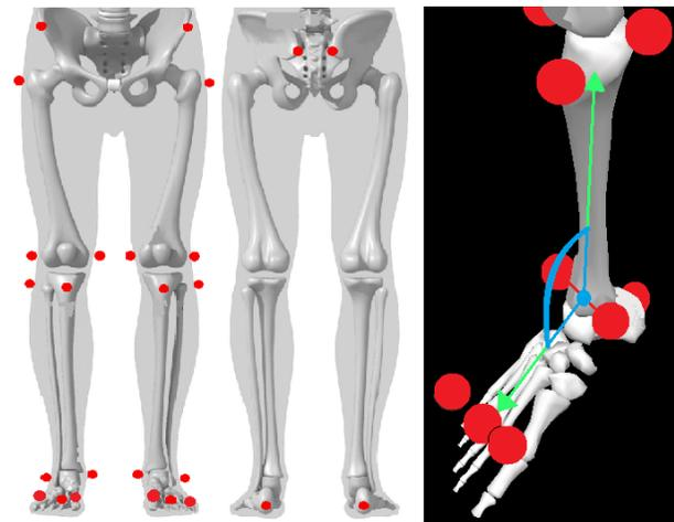
Figure 7: *Left*: Marker model from Leardini et al. [37]. The markers are shown as red dots. The foot markers were placed on the shoes. At least three markers are placed on each segment. *Right*: Ankle angle [38] (blue) used to determine the feedback parameter for biofeedback.
