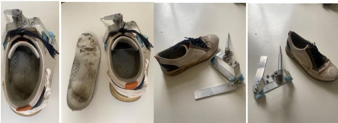
The length of the rod can be adjusted by replacing the upper threaded wire with one of a different length. The frame can be attached to a different shoe, therefore accommodating for different foot lengths.
