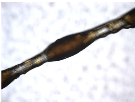
Figure 2.24: An image of a compartmented alginate fibre encapsulating rejuvenator captured by optical microscope. Plane polarized light imaging. The field of view is approximately 3mm [36].
