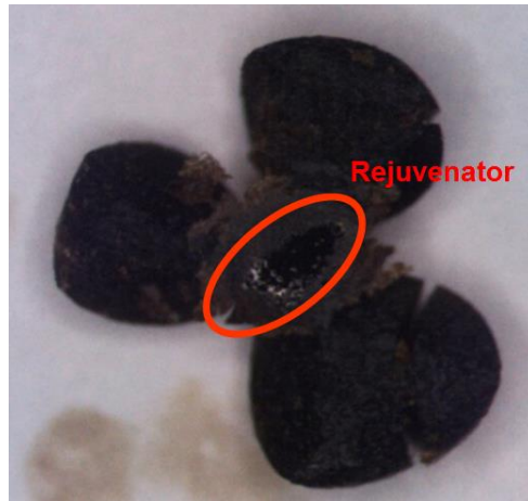
Figure 4.11: Rejuvenator flowing out of a crashed calcium alginate capsule (A/R ratio of 30/70) after the compressive test.
