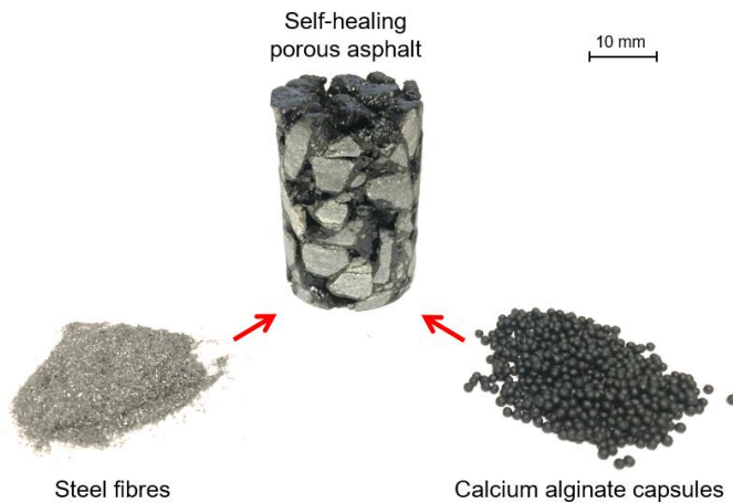
Figure 6.2: Steel fibres and calcium alginate capsules used in self-healing porous asphalt.
