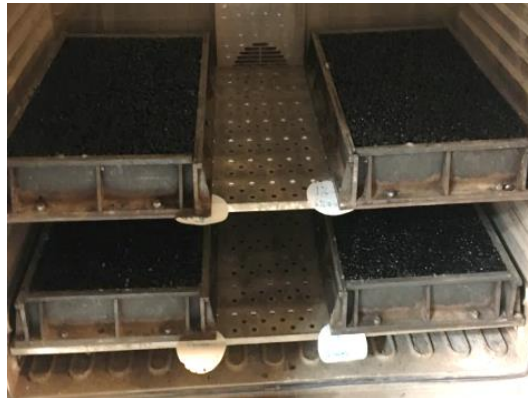
Figure 5.2: Asphalt mortar mixture filled in silicon container before the ageing process.
