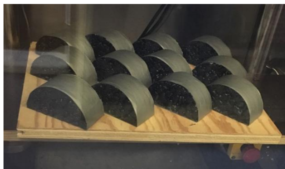
Figure 5.10: Healing of the fractured SCB samples in a temperature chamber
