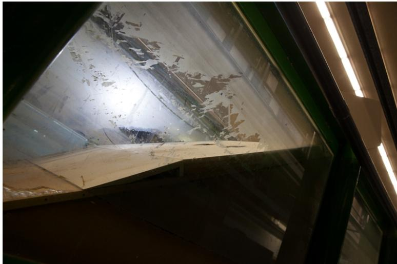
Figure C.6: Transition between the embedded cube and slope. Transition angle = 1:6
