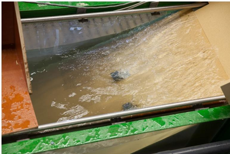
Figure C.3: Wave run-up for exposed cubes. No movement
