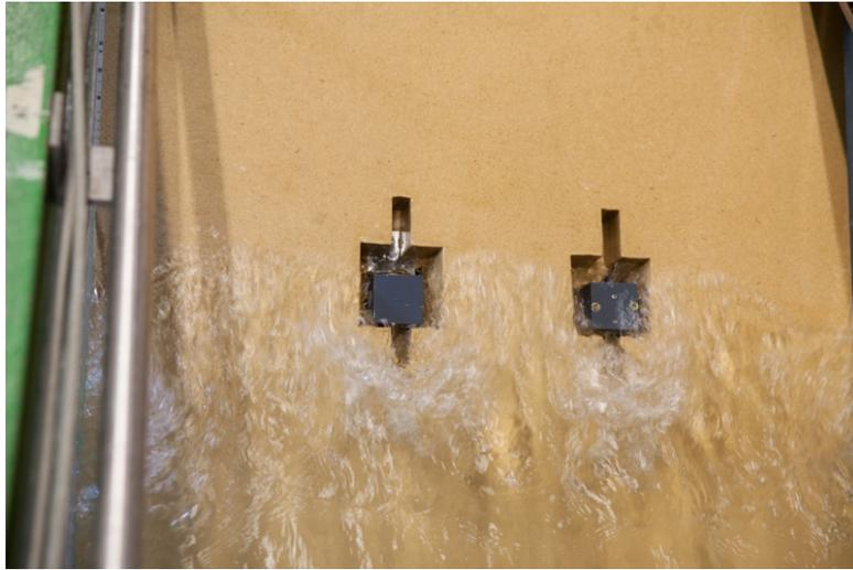
Figure C.5: Wave run-up for the embedded cubes
