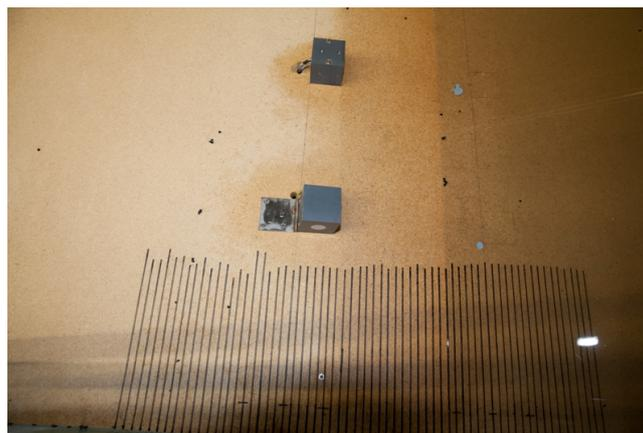
Figure 4.10: Placement of cube measuring pressure (upper cube) and cube measuring accelerations (lower cube)
