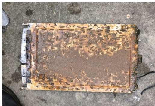
Figure SI 7.1 Iron precipitation on an aeration sampling plate
