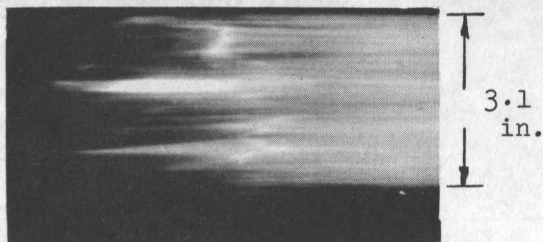
(f) Observed Wave Shape at r/R=0.5 (Shot No. 1); Streaks Indicate Jets
