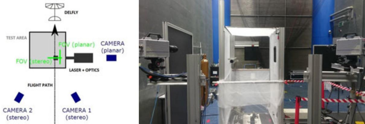
Fig. 5. Top view schematic of the test arrangement (left); setup for the stereoscopic PIV measurements (right).
