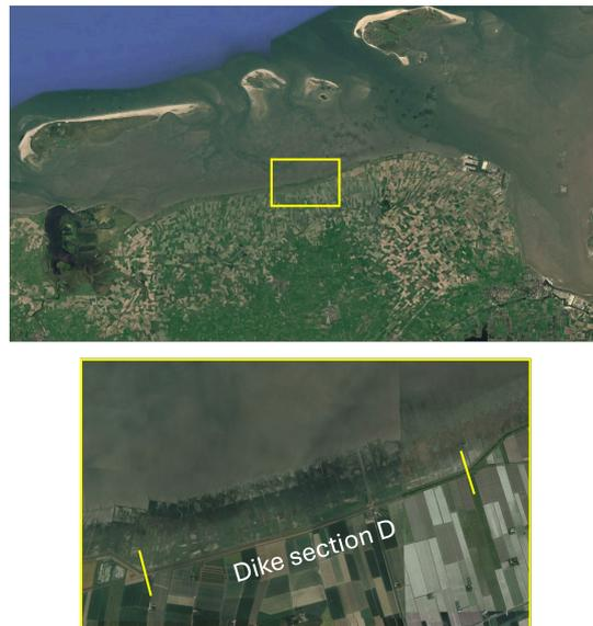
Figure 6.1: Section D, the dike section with highest probability of failure (Google, 2025)
