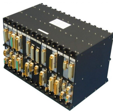
Figure 4.23: The ICDE-NG OBC developed by Airbus Defense and Space [7].
