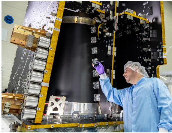
Figure 4.29: Satellite using a honeycomb sandwich structure [18].
