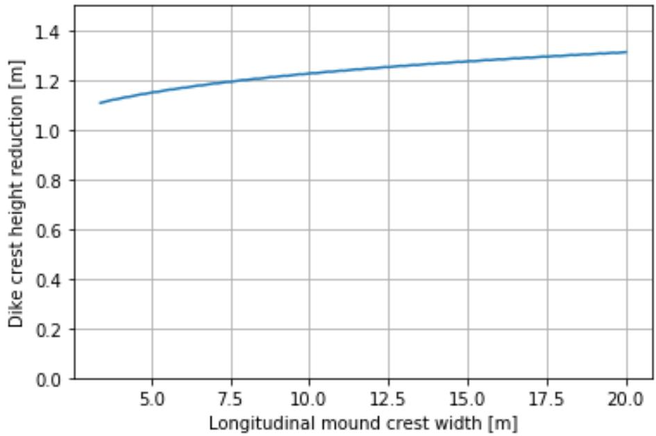
Figure D-19 Dike crest height reduction based on crest width of longitudinal mound for location Waal\_09
