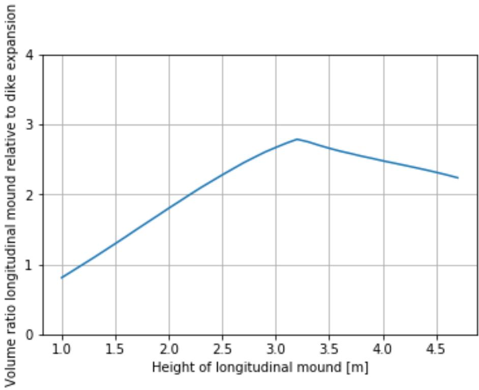
Figure D-17 Volume ratio based on crest height of longitudinal mound for location Rijn\_01
