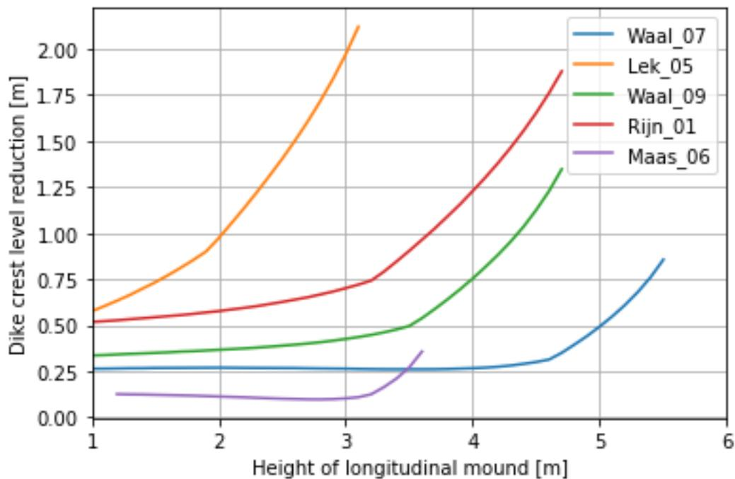
Figure 40 Dike crest height reduction based on height of longitudinal mound for all locations
