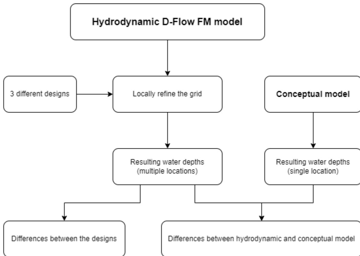
Figure 17 Flow chart for the D-Flow FM model
