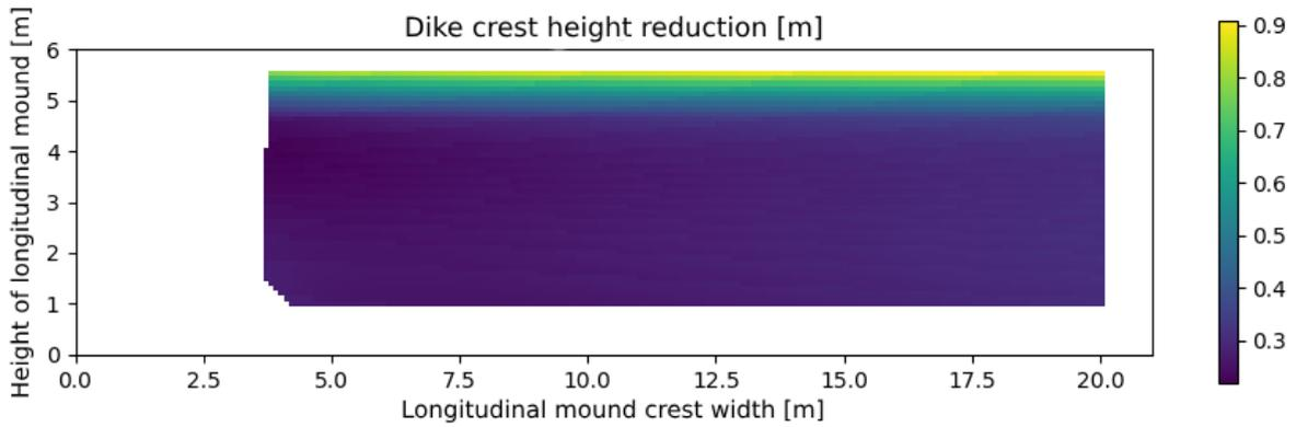
Figure D-3 Dike crest height in metres for all combination of width and length of the longitudinal mound for location Waal\_07
