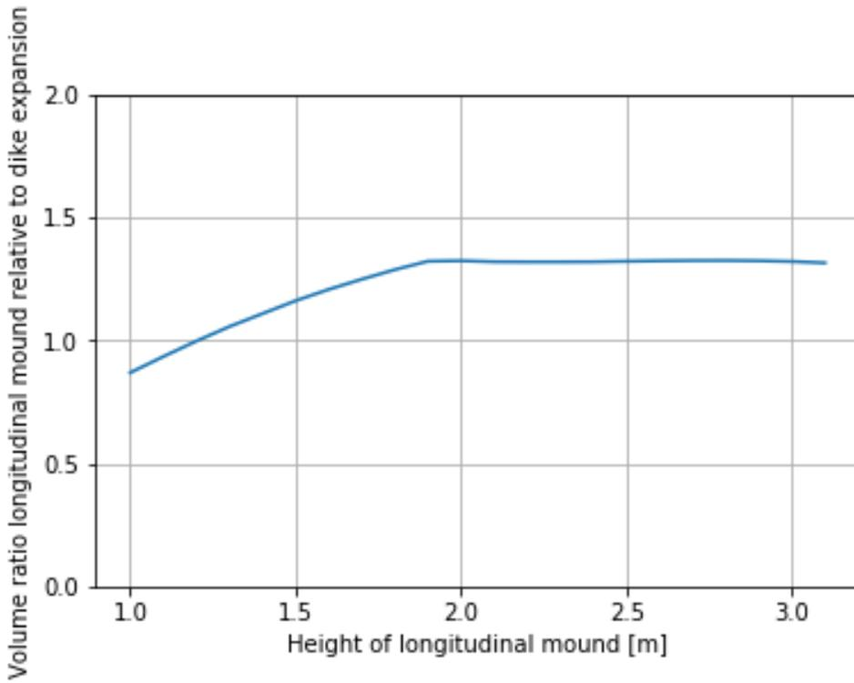
Figure D-11 Volume ratio based on crest height of longitudinal mound for location Lek\_05
