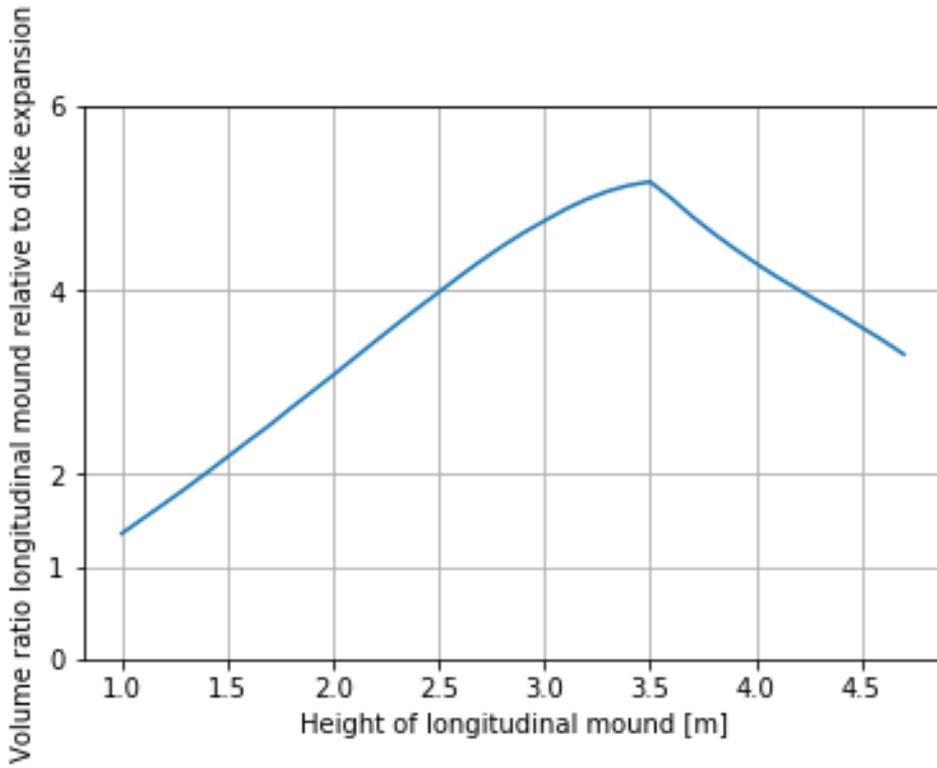
Figure D-23 Volume ratio based on crest height of longitudinal mound for location Waal\_09
