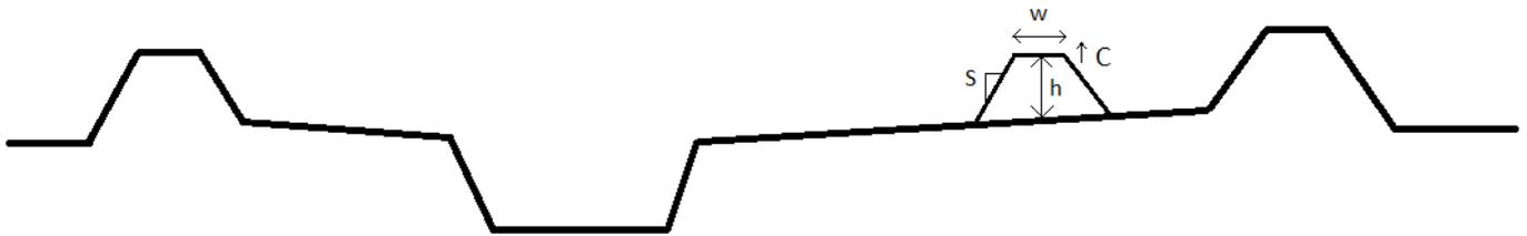
Figure 14 Design variables for the longitudinal mound
