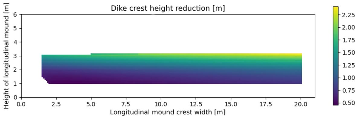
Figure D-9 Dike crest height in metres for all combination of width and length of the longitudinal mound for location Lek\_05
