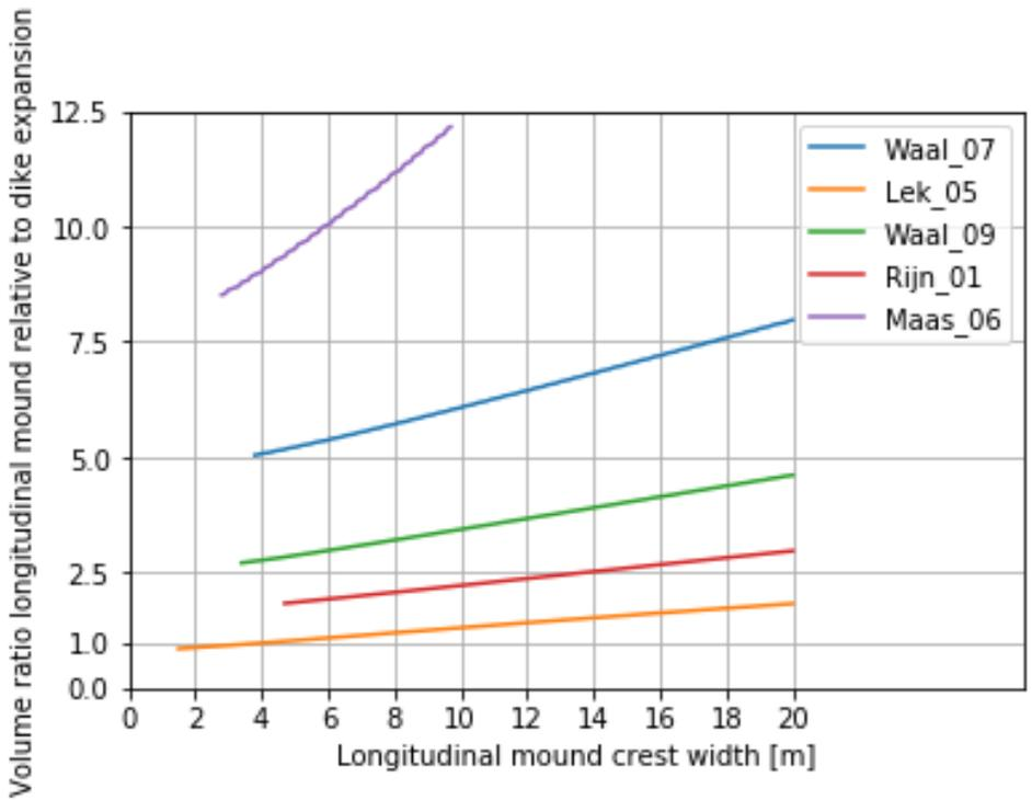
Figure D-33 Volume ratio based on crest width of longitudinal mound for all locations
