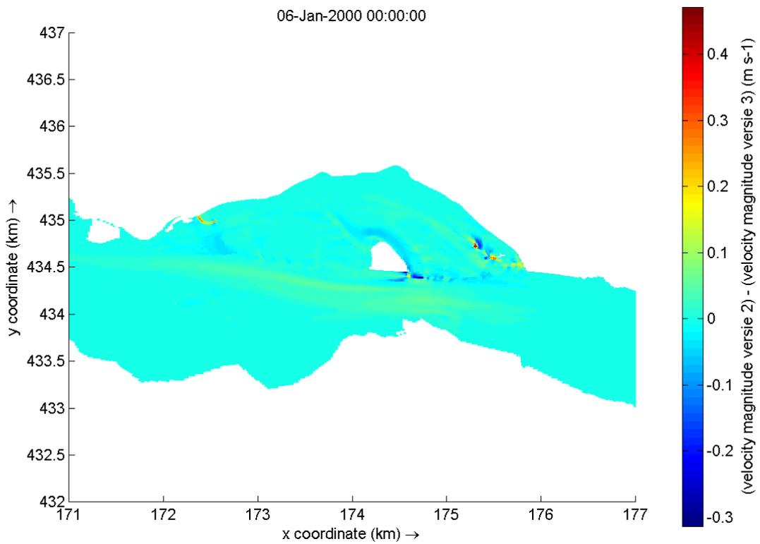
Figure F-13 Differences in flow velocity between the variant 1 and variant 2. Red indicates a higher flow velocity and dark blue a lower flow velocity in variant 2 than in variant 3
