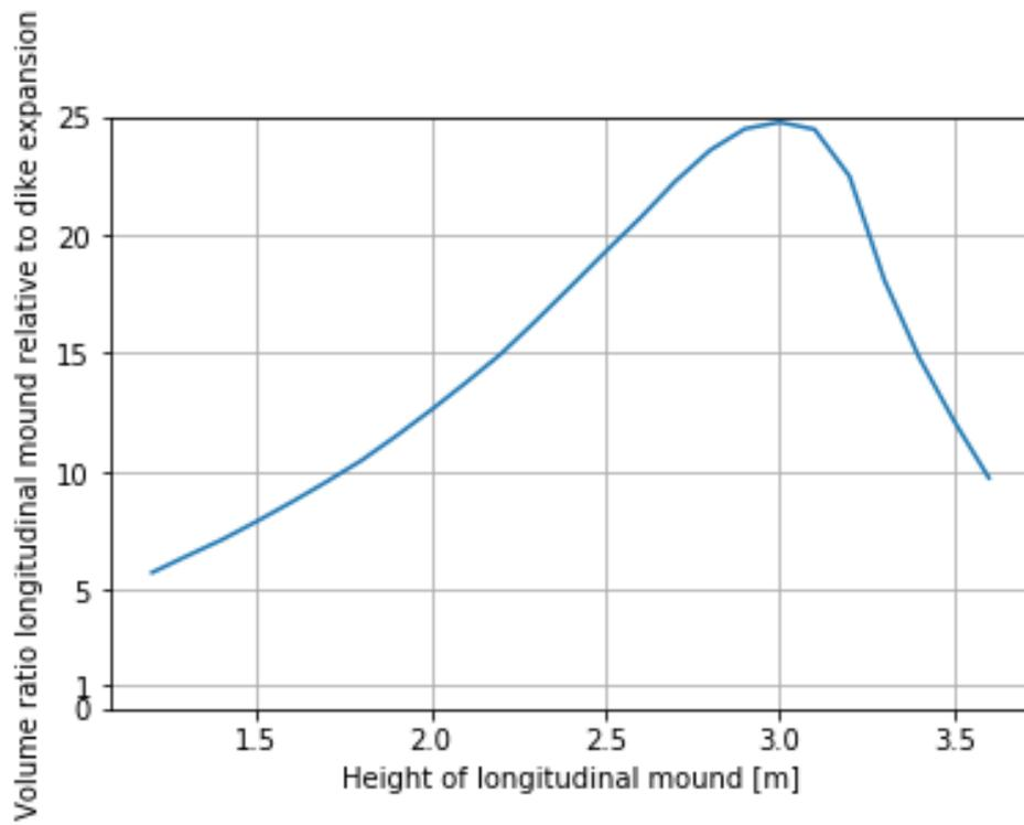
Figure D-29 Volume ratio based on crest height of longitudinal mound for location Maas\_06
