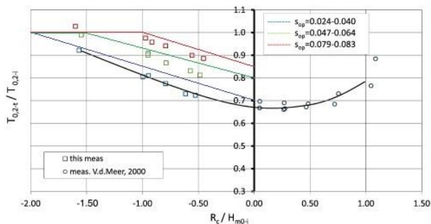
Figure 16 Reduction of spectral wave period based on the relative freeboard (Carevic et al. 2013). Includes conservative approximations based on the wave steepness.
