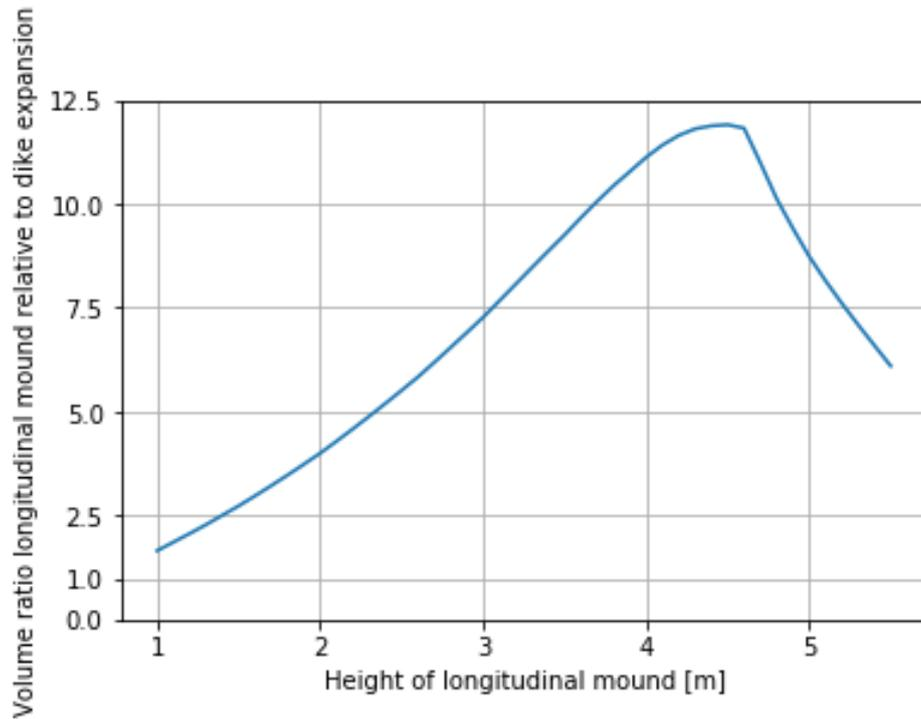
Figure 38 Volume ratio based on crest height of longitudinal mound
