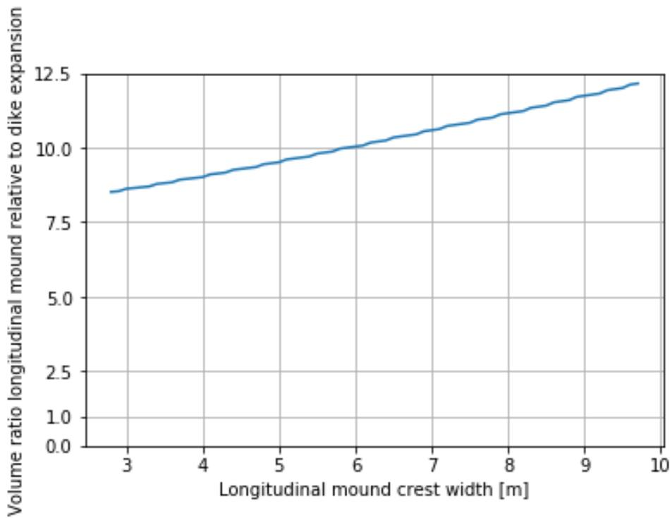
Figure D-28 Volume ratio based on crest width of longitudinal mound for location Maas\_06
