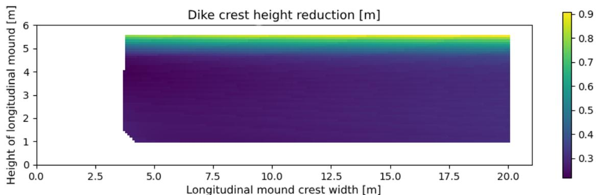
Figure 36 Dike crest height in metres for all combinations of width and length of the longitudinal mound
