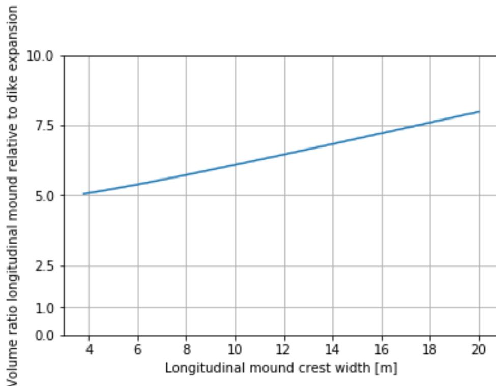
Figure 37 Volume ratio based on crest width of longitudinal mound
