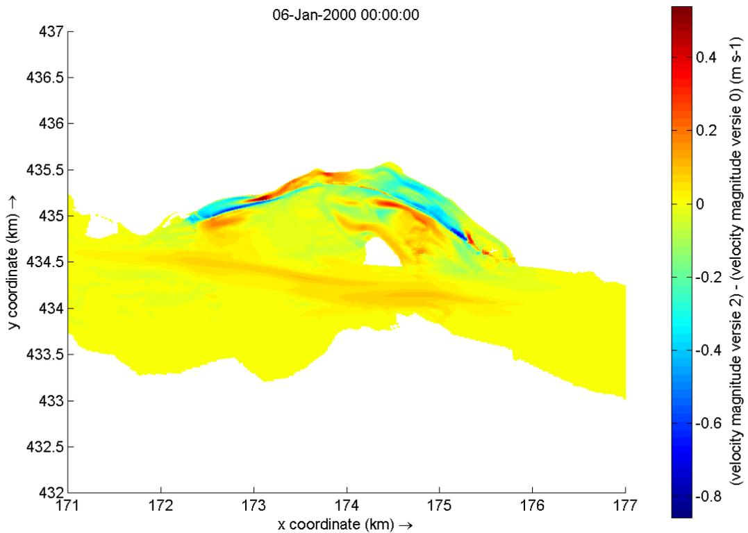
Figure F-9 Differences in flow velocity between the original situation and variant 2. Red indicates an increase in flow velocity and dark blue a decrease in flow velocity
