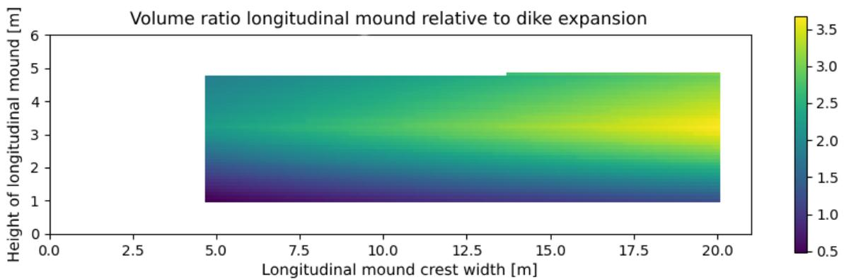
Figure D-18 Volume ratio between longitudinal mound and dike expansion for all combinations of the longitudinal mound for location Rijn\_01
