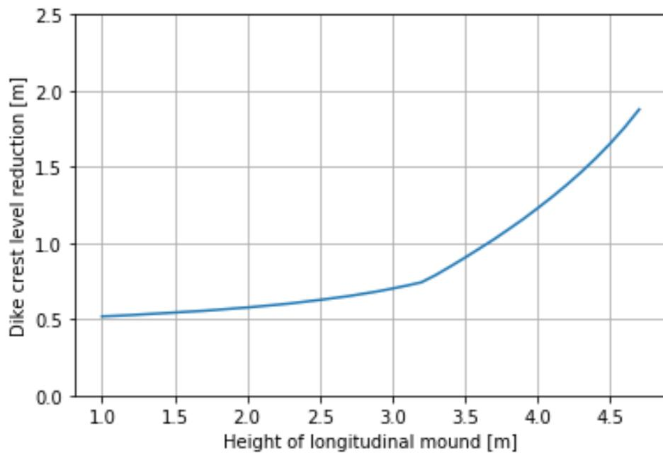
Figure D-14 Dike crest height reduction based on crest height of longitudinal mound for location Rijn\_01
