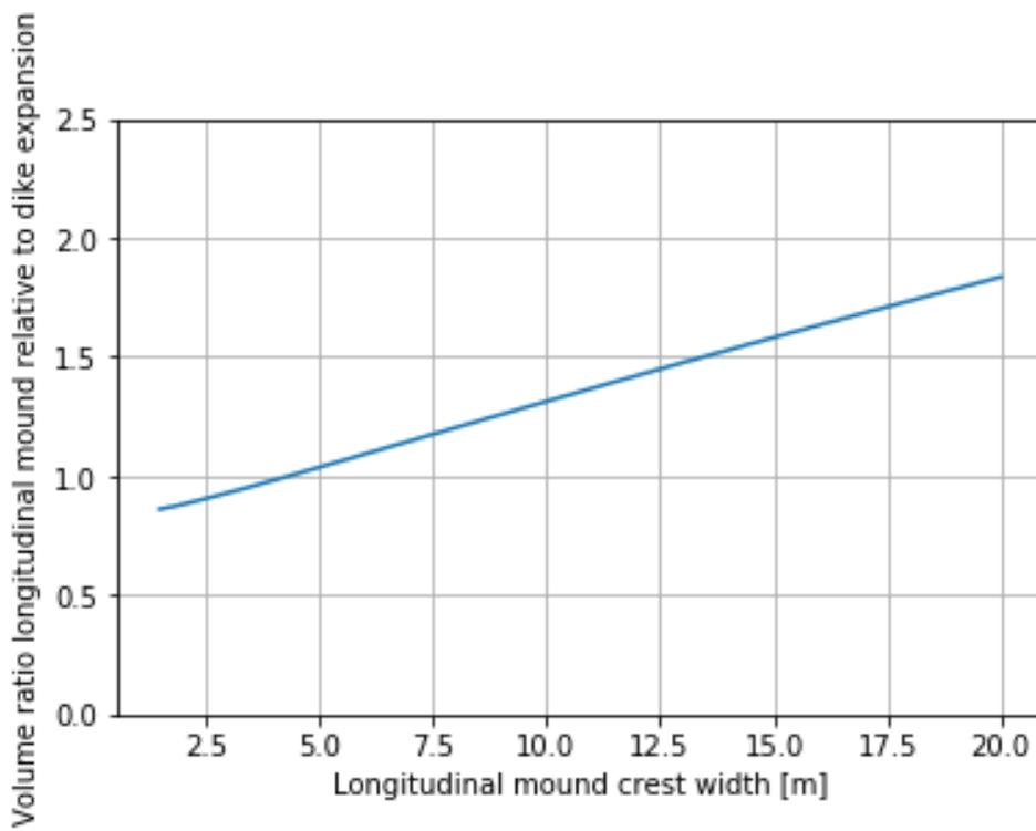
Figure D-10 Volume ratio based on crest width of longitudinal mound for location Lek\_05
