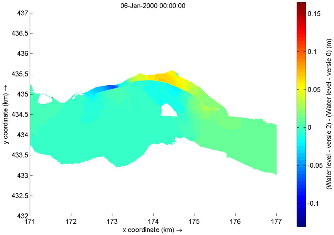
Figure F-2 Water level differences between the original situation and variant 2. Red indicates a water level increase and dark blue a water level decrease
