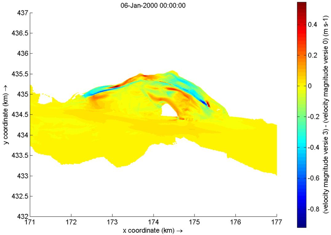
Figure F-10 Differences in flow velocity between the original situation and variant 1. Red indicates an increase in flow velocity and dark blue a decrease in flow velocity
