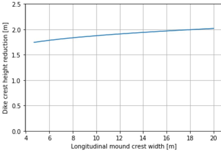
Figure D-13 Dike crest height reduction based on crest width of longitudinal mound for location Rijn\_01
