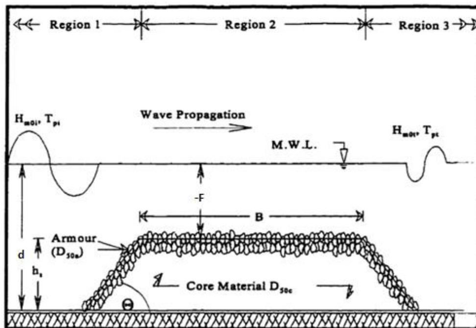
Figure 6 Example of a rubble mound submerged breakwater from Seabrook (1997).
