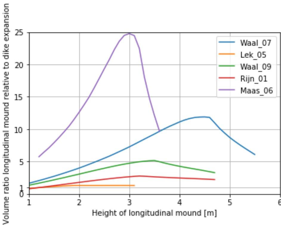
Figure D-34 Volume ratio based on crest height of longitudinal mound for all locations
