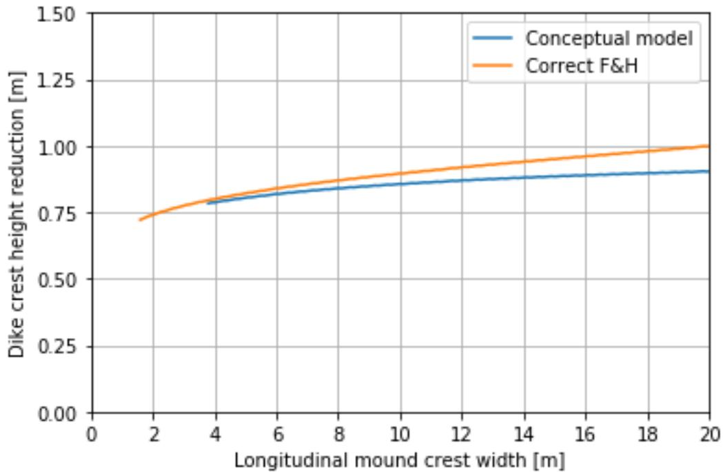
Figure D-35 Difference between the conceptual model and the correct Friebel and Harris formula
