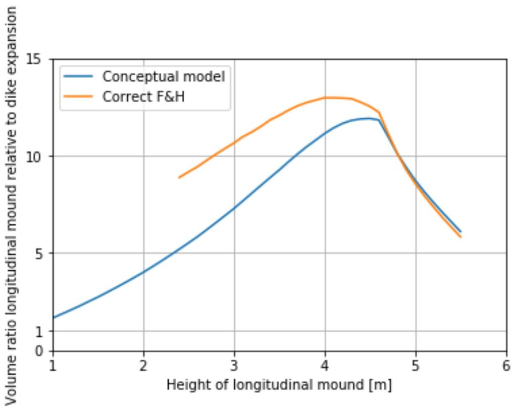
Figure 49 Difference between the conceptual model and the correct Friebel and Harris formula
