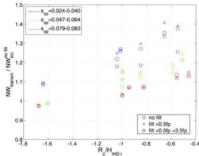
Figure 7 Increase in number of transmitted waves based on wave steepness and relative freeboard (Carevic et al. 2013)
