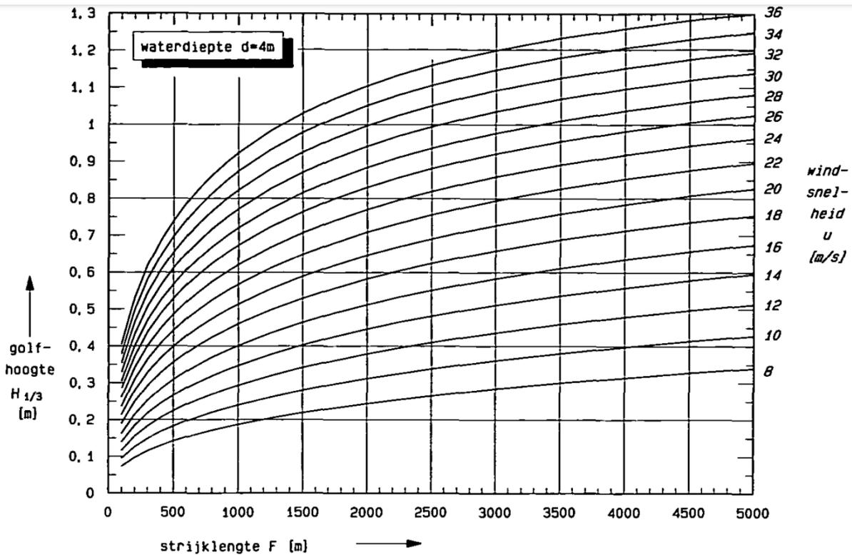
Figure 4 Example of Bretschneider wave growth curve. Water depth of 4 metres. (TAW, 1989)
