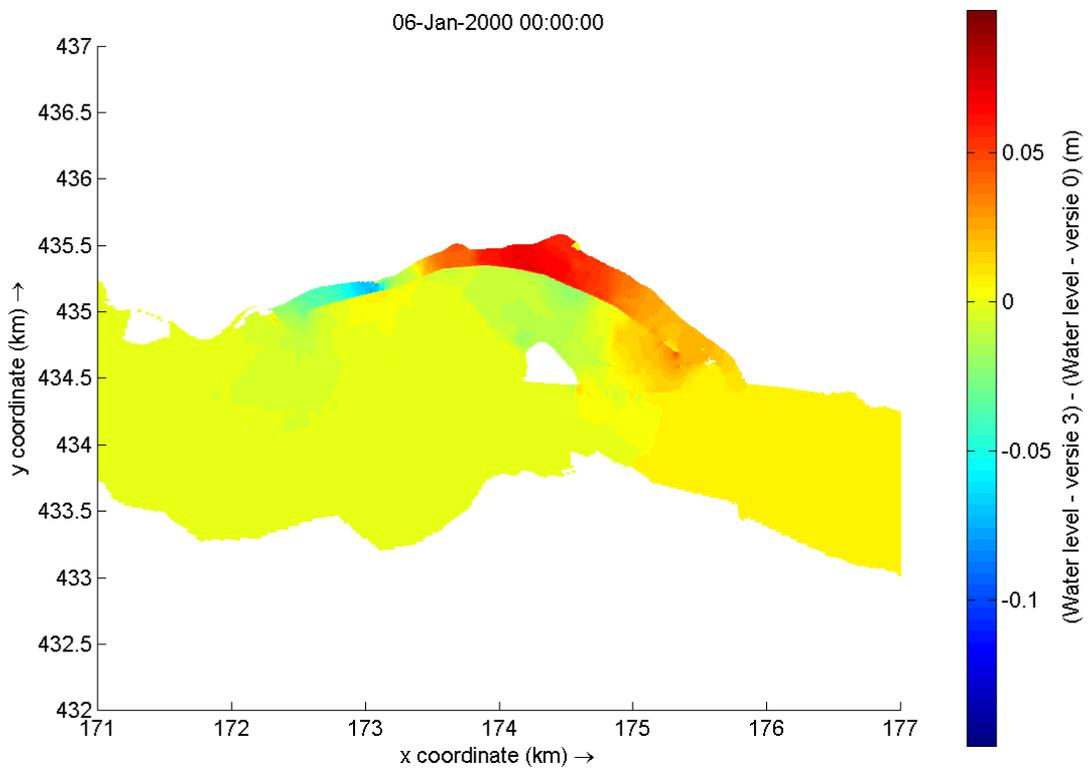
Figure F-3 Water level differences between the original situation and variant 3. Red indicates a water level increase and dark blue a water level decrease
