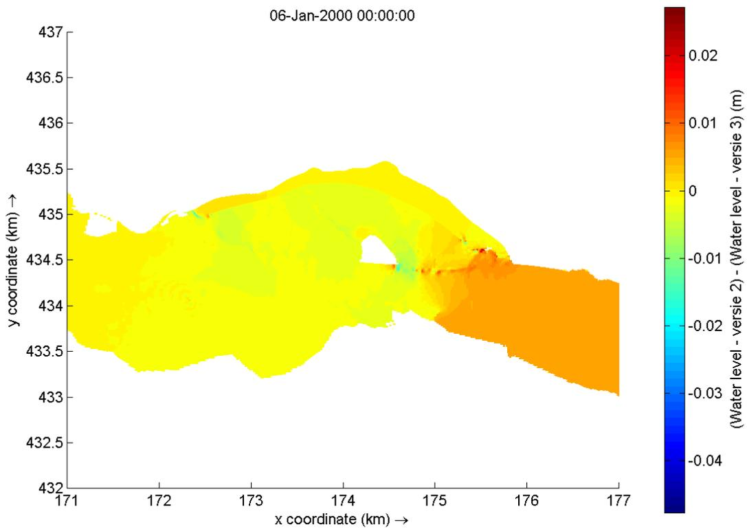
Figure F-6 Water level differences between variant 1 and variant 2. Red indicates a higher water level and dark blue a lower water level for variant 2 than variant 3
