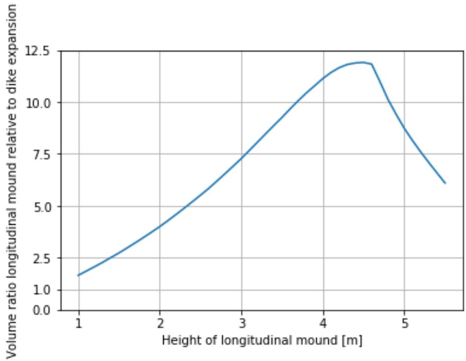
Figure D-5 Volume ratio based on crest height of longitudinal mound for location Waal\_07
