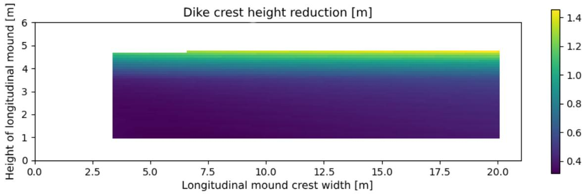
Figure D-21 Dike crest height in metres for all combination of width and length of the longitudinal mound for location Waal\_09
