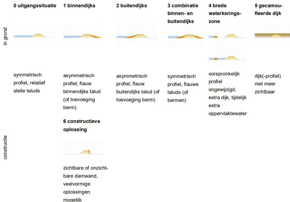
Figure 2 Cross sections of the different types of deltadikes. (In Dutch, Klijn & Bos, 2010)
