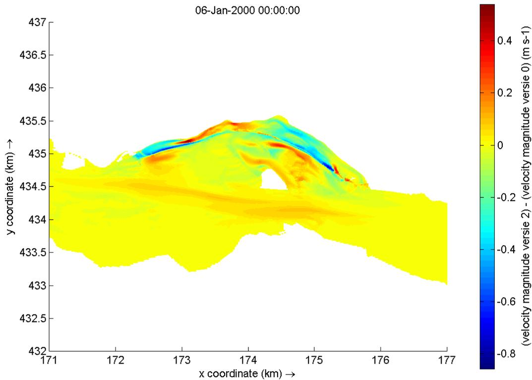
Figure 47 Flow velocity increase from variant 0 to variant 2
