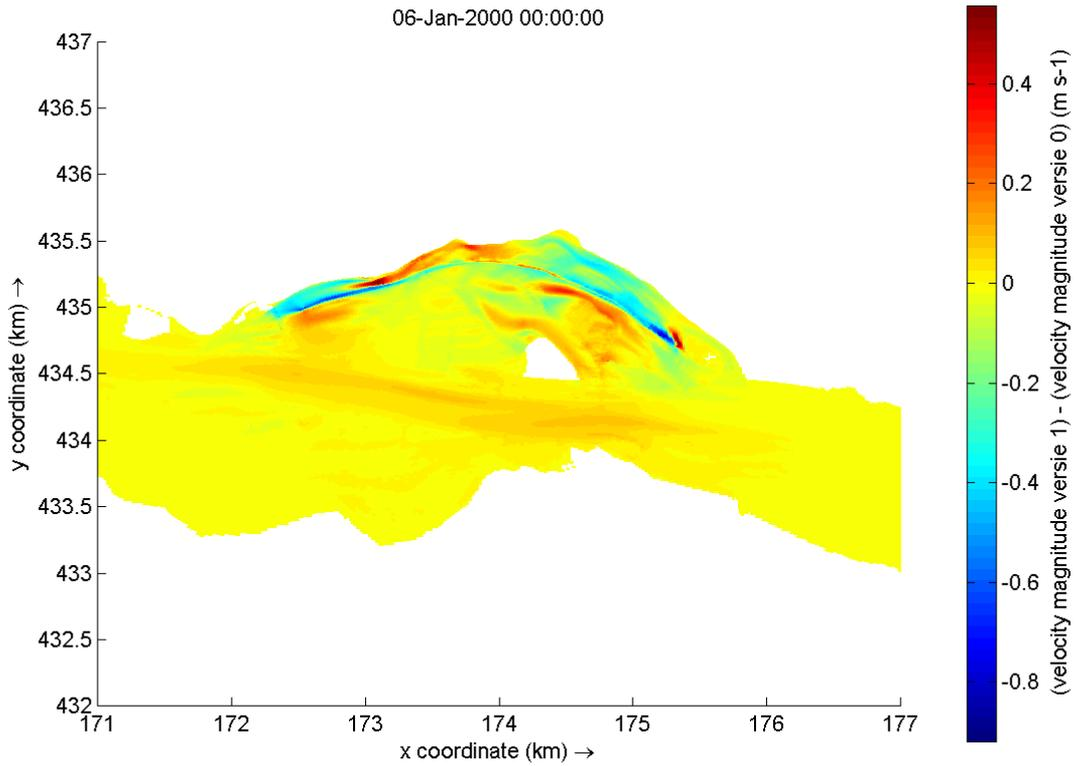
Figure F-8 Differences in flow velocity between the original situation and variant 1. Red indicates an increase in flow velocity and dark blue a decrease in flow velocity
