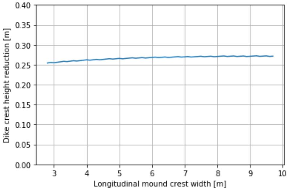
Figure D-25 Dike crest height reduction based on crest width of longitudinal mound for location Maas\_06
