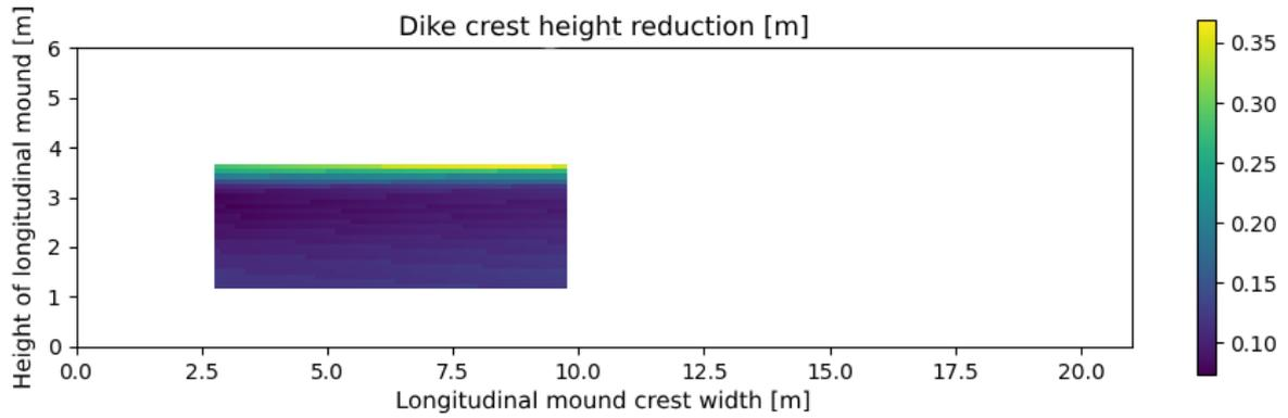
Figure D-27 Dike crest height in metres for all combination of width and length of the longitudinal mound for location Maas\_06
