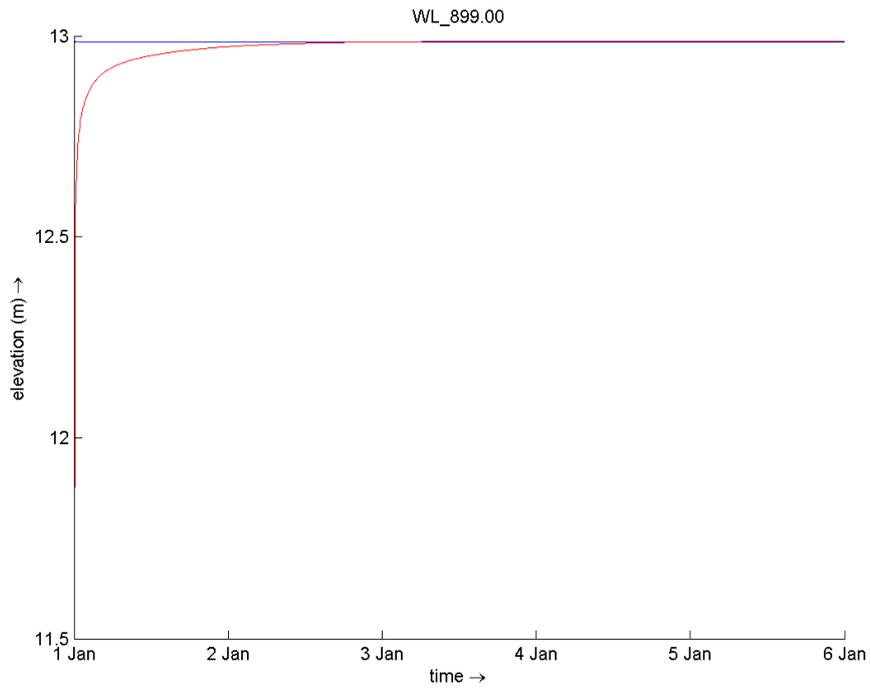
Figure 42 Water levels at WL\_899 over the entire simulation period for both the original and new grid.
