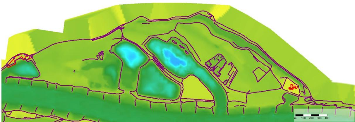
Figure 19 Area of Waal\_07 with the bottom profile and with the D-Flow FM fixed weirs in purple
