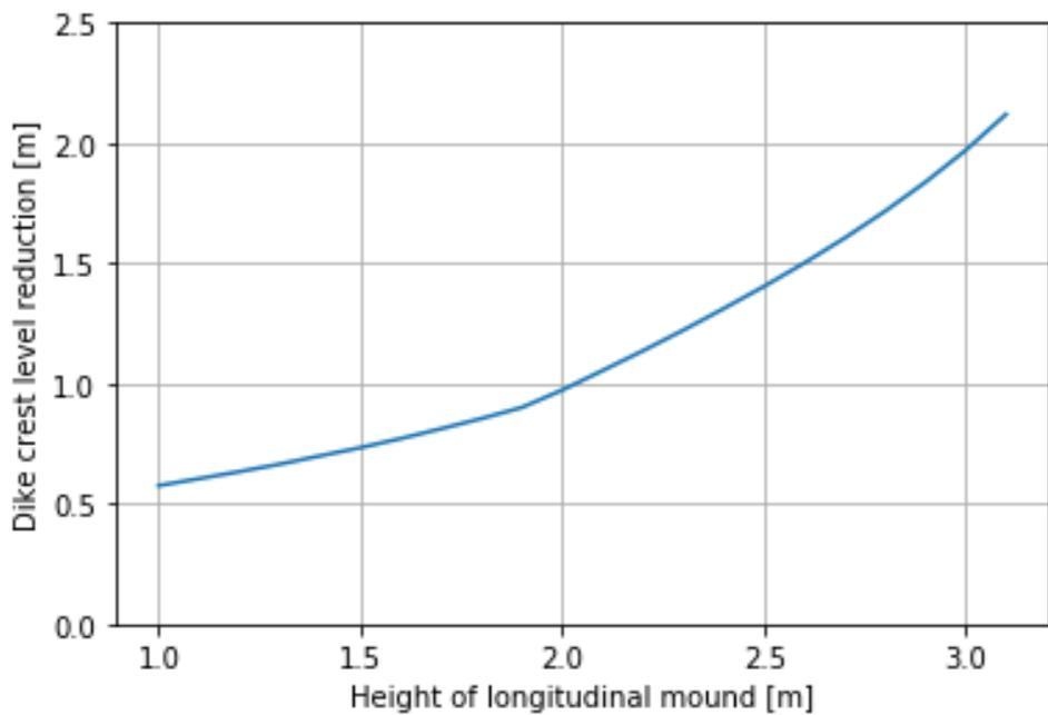
Figure D-8 Dike crest height reduction based on crest height of longitudinal mound for location Lek\_05
