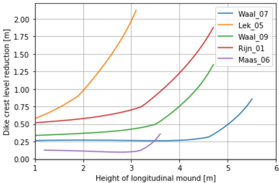
Figure D-32 Dike crest height reduction based on crest height of longitudinal mound for all locations
