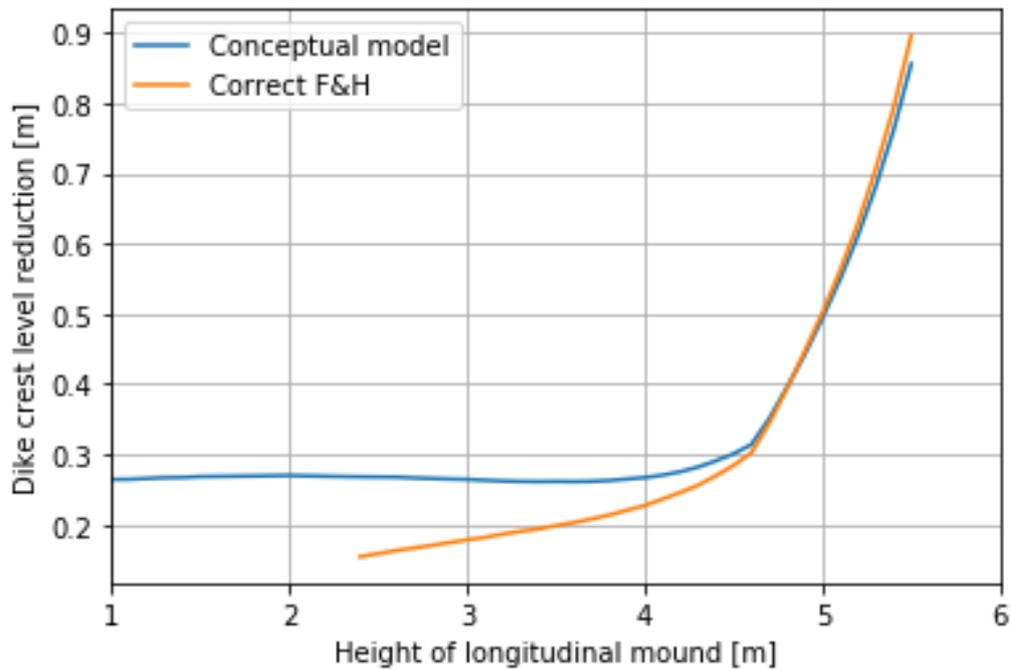
Figure 48 Difference between the conceptual model and the correct Friebel and Harris formula
