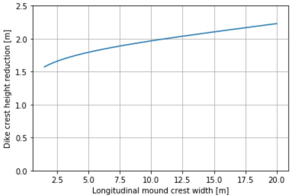
Figure D-7 Dike crest height reduction based on crest width of longitudinal mound for location Lek\_05
