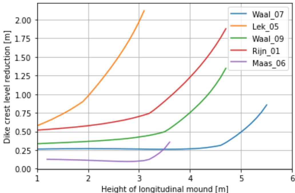
Figure 40 Dike crest height reduction based on height of longitudinal mound for all locations
