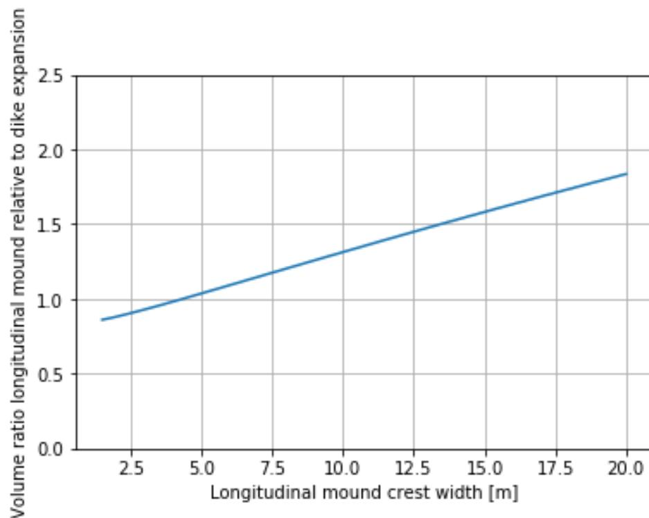
Figure D-10 Volume ratio based on crest width of longitudinal mound for location Lek\_05
