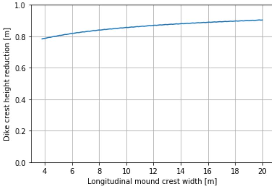
Figure D-1 Dike crest height reduction based on crest width of longitudinal mound for location Waal\_07
