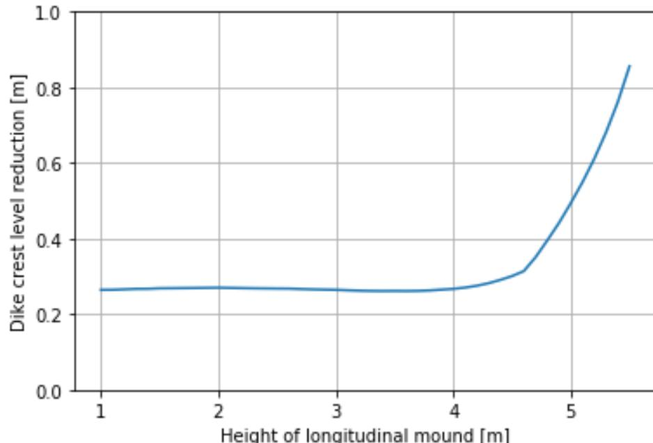
Figure D-2 Dike crest height reduction based on crest height of longitudinal mound for location Waal\_07
