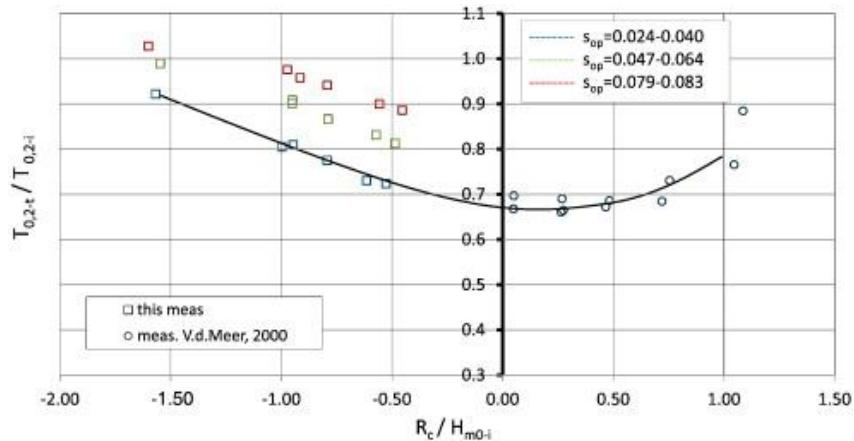
Figure 8 Reduction of the wave period based on the relative freeboard (Carevic et al. 2013)
