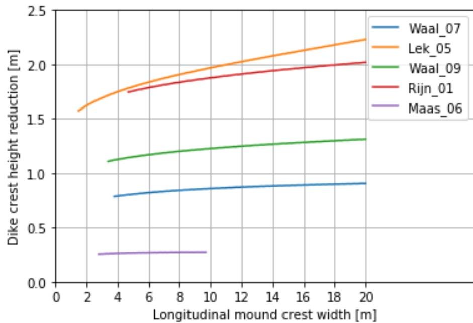
Figure D-31 Dike crest height reduction based on crest height of longitudinal mound for all locations
