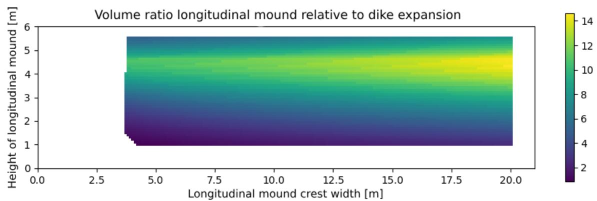
Figure D-6 Volume ratio between longitudinal mound and dike expansion for all combinations of the longitudinal mound for location Waal\_07
