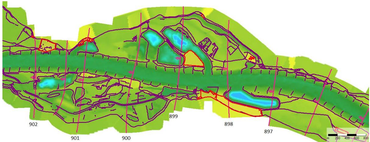
Figure 41 Original topography at location Waal\_07 including the cross-section measurement locations.
