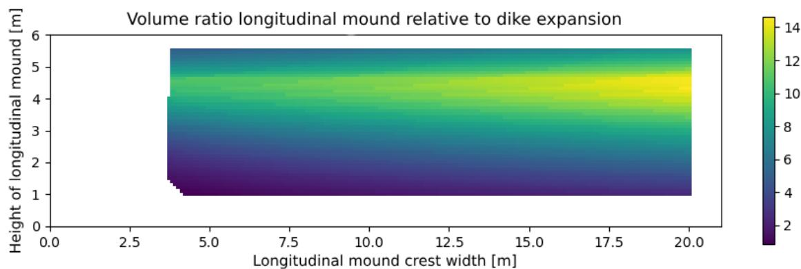
Figure 39 Volume ratio between longitudinal mound and dike expansion for all combinations of the longitudinal mound
