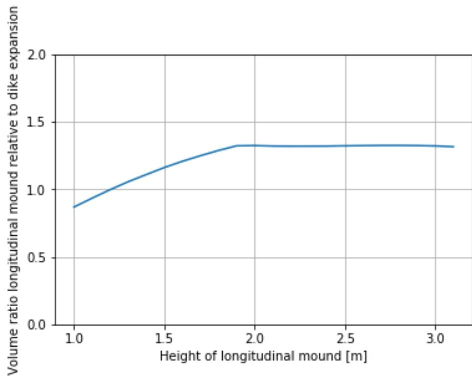
Figure D-11 Volume ratio based on crest height of longitudinal mound for location Lek\_05
