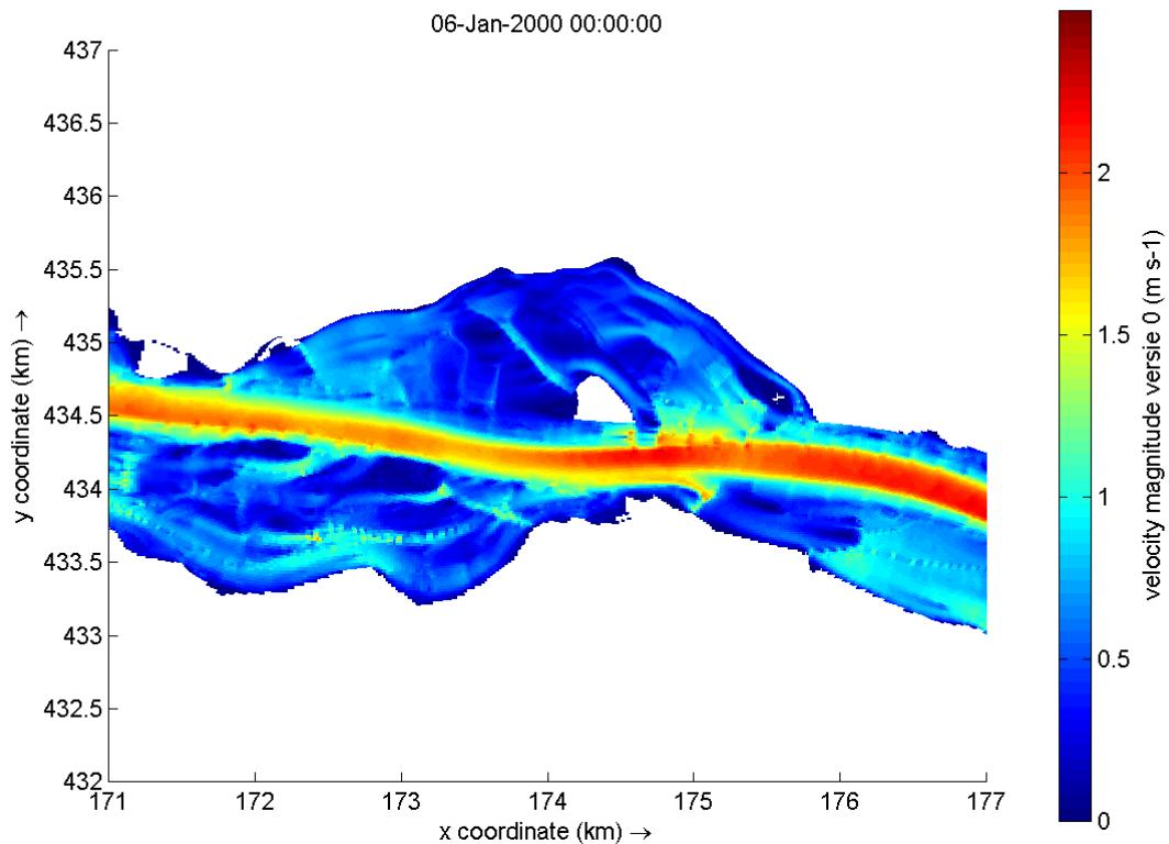
Figure F-7 Flow velocities in the channel and on the floodplain in the original situation
