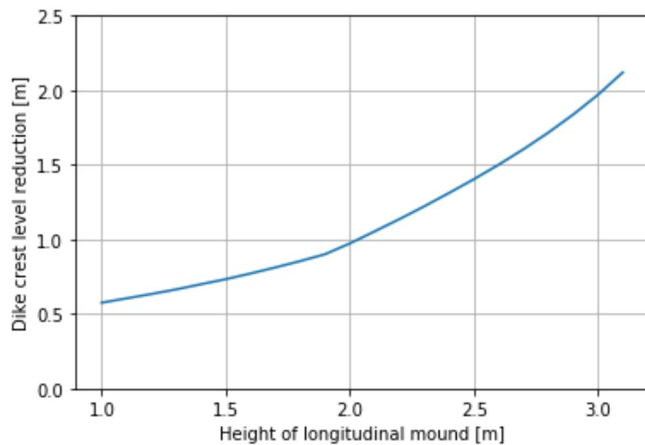
Figure D-8 Dike crest height reduction based on crest height of longitudinal mound for location Lek\_05
