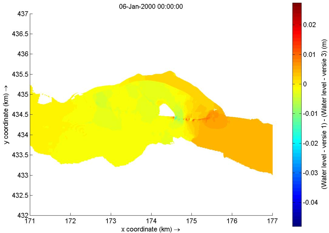
Figure F-5 Water level differences between variant 1 and variant 2. Red indicates a higher water level and dark blue a lower water level for variant 1 than variant 3
