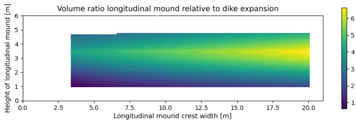
Figure D-24 Volume ratio between longitudinal mound and dike expansion for all combinations of the longitudinal mound for location Waal\_09
