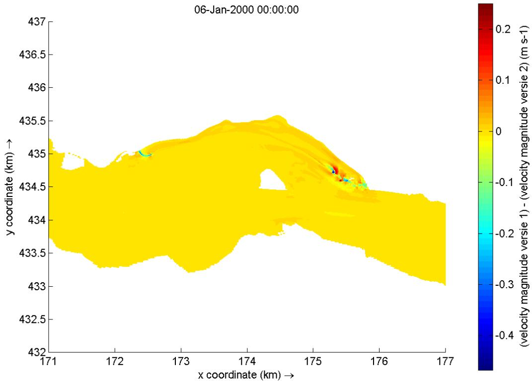
Figure F-11 Differences in flow velocity between the variant 1 and variant 2. Red indicates a higher flow velocity and dark blue a lower flow velocity in variant 1 than in variant 2
