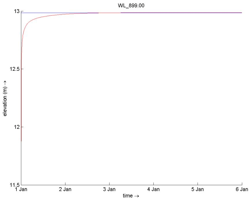
Figure 42 Water levels at WL\_899 over the entire simulation period for both the original and new grid.
