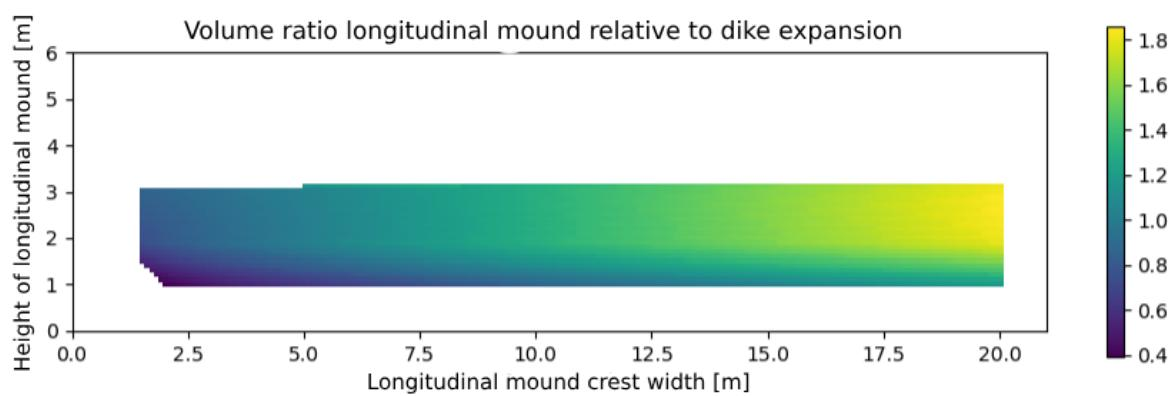
Figure D-12 Volume ratio between longitudinal mound and dike expansion for all combinations of the longitudinal mound for location Lek\_05
