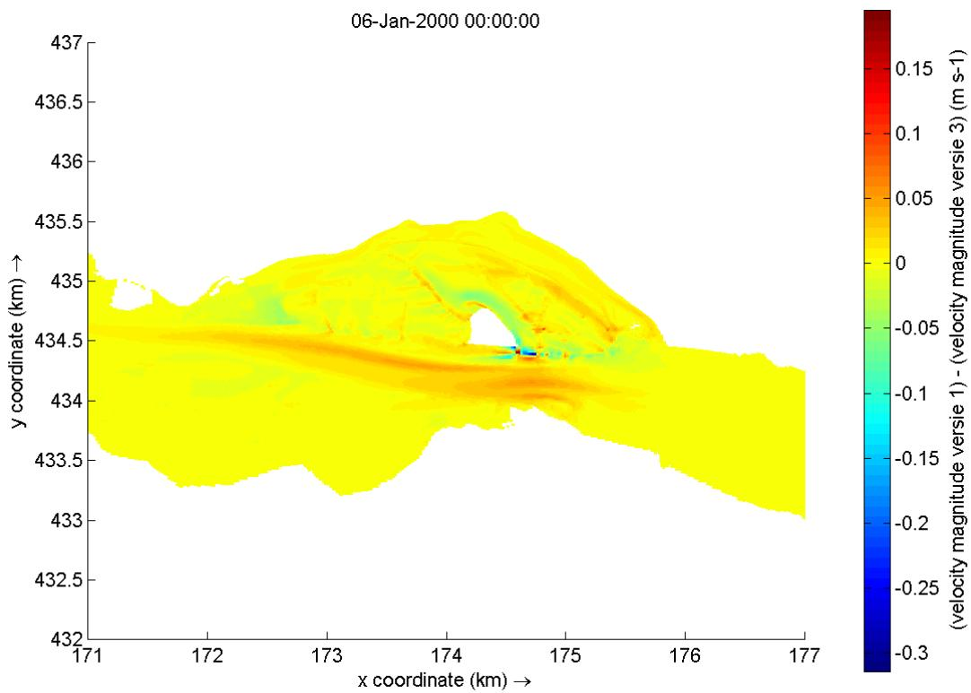
Figure F-12 Differences in flow velocity between the variant 1 and variant 2. Red indicates a higher flow velocity and dark blue a lower flow velocity in variant 1 than in variant 3
