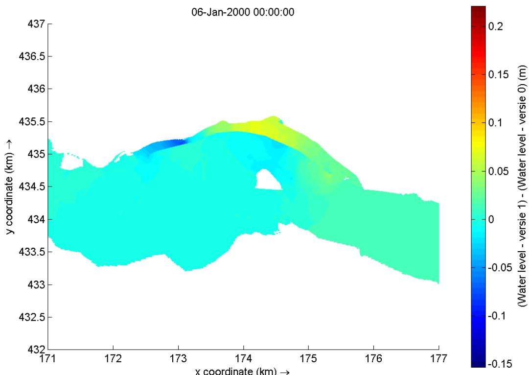
Figure F-1 Water level differences between the original situation and variant 1. Red indicates a water level increase and dark blue a water level decrease
