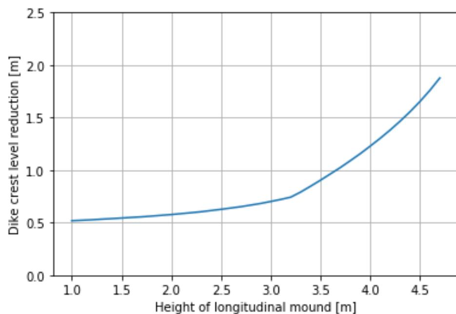
Figure D-14 Dike crest height reduction based on crest height of longitudinal mound for location Rijn\_01
