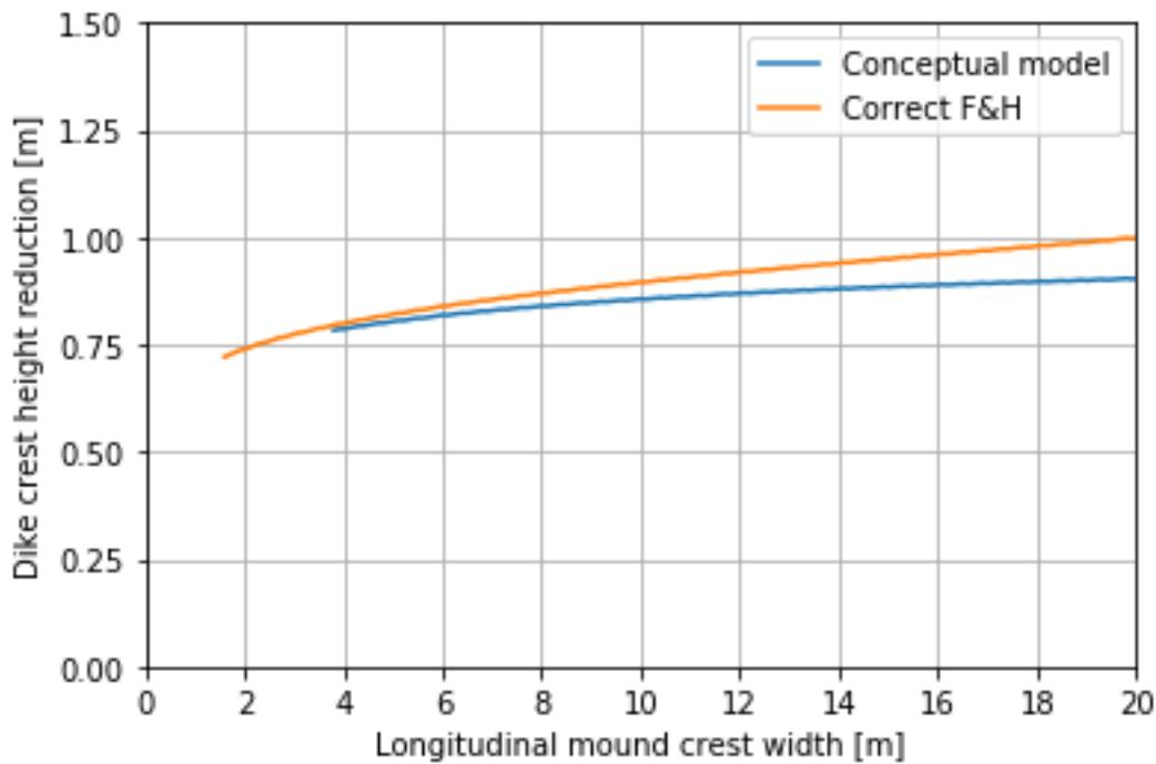
Figure D-35 Difference between the conceptual model and the correct Friebel and Harris formula
