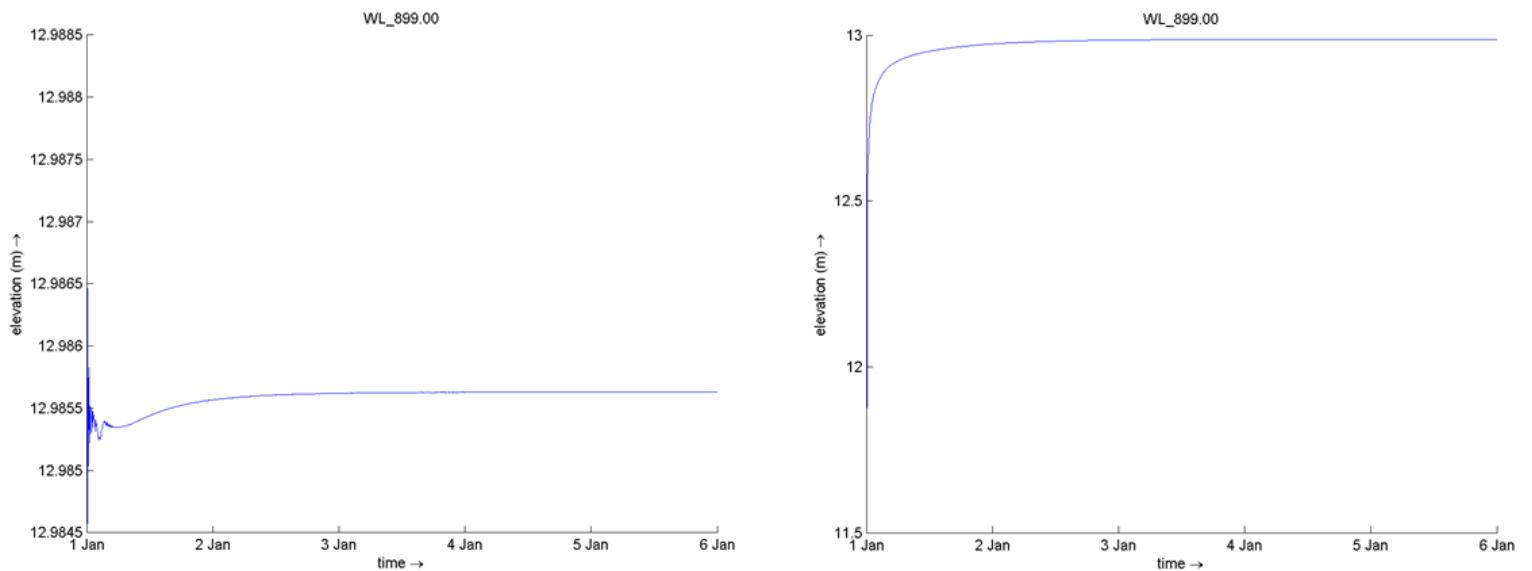
Figure 43 Water levels at WL\_899 over the entire simulation period. Left side: original grid. Right side: new grid.
