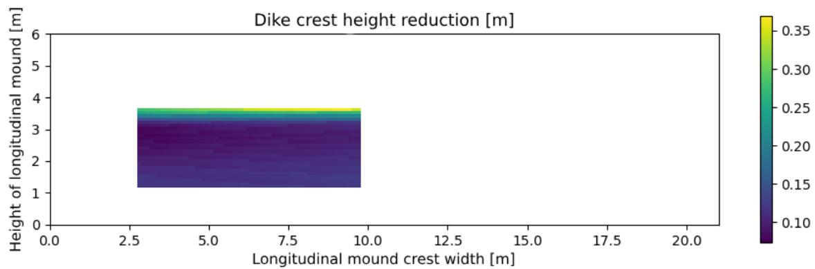
Figure D-27 Dike crest height in metres for all combination of width and length of the longitudinal mound for location Maas\_06
