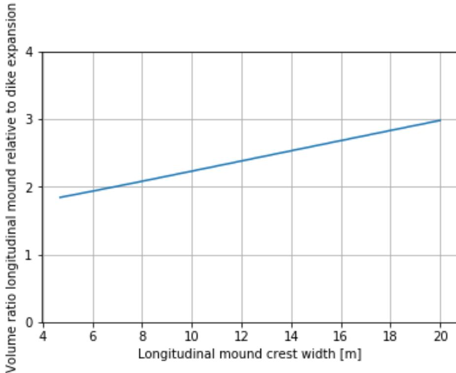
Figure D-16 Volume ratio based on crest width of longitudinal mound for location Rijn\_01
