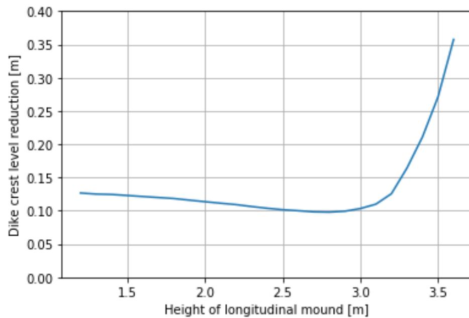
Figure D-26 Dike crest height reduction based on crest height of longitudinal mound for location Maas\_06
