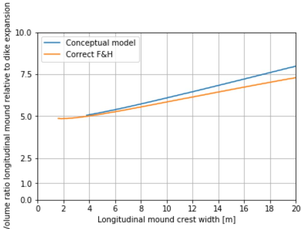
Figure D-36 Difference between the conceptual model and the correct Friebel and Harris formula
