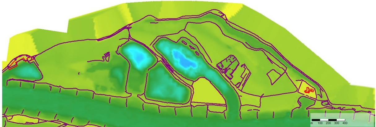
Figure 19 Area of Waal\_07 with the bottom profile and with the D-Flow FM fixed weirs in purple
