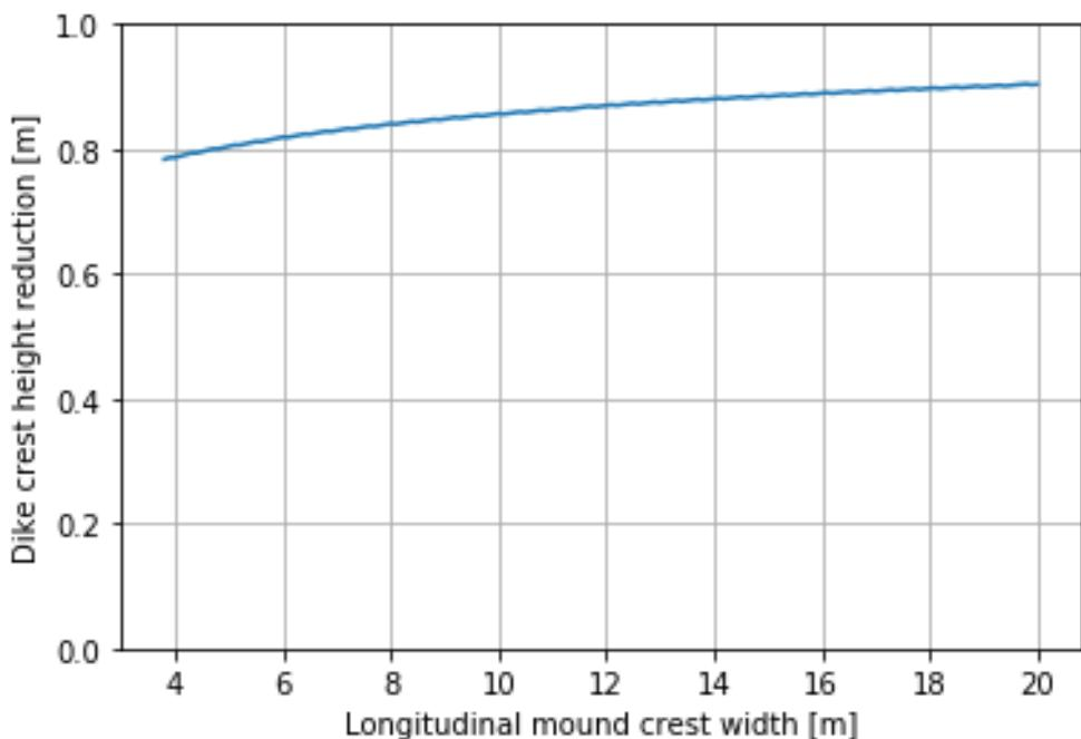
Figure 34 Dike crest height reduction based on crest width of longitudinal mound
