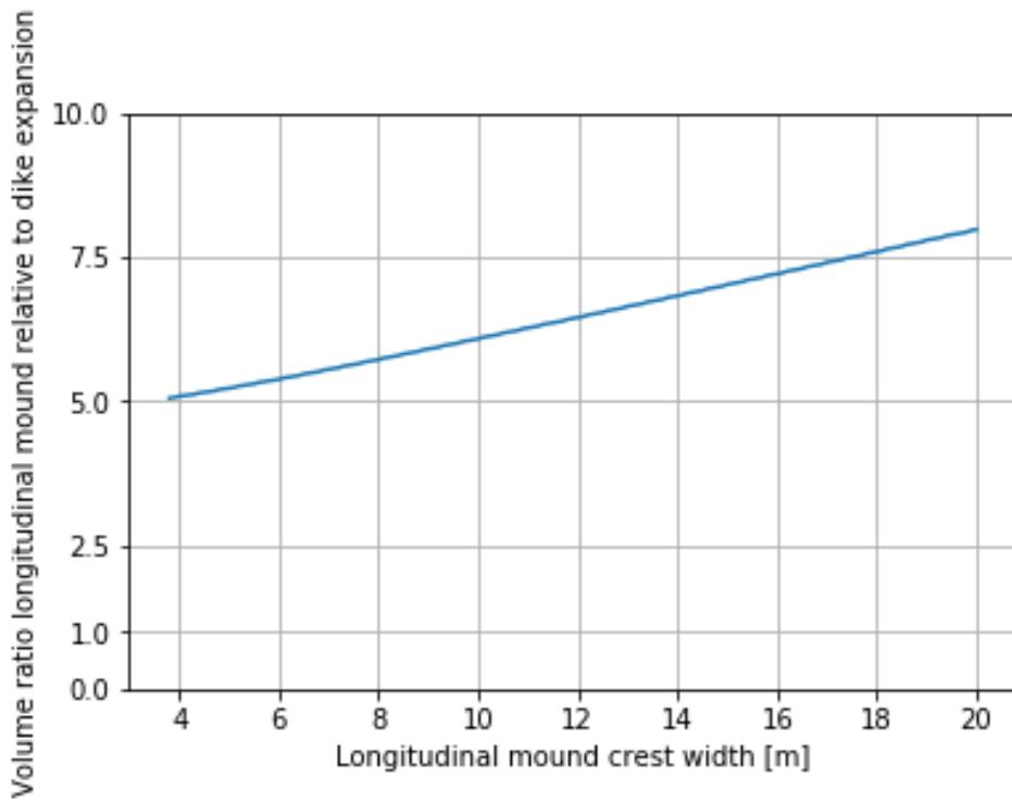
Figure D-4 Volume ratio based on crest width of longitudinal mound for location Waal\_07
