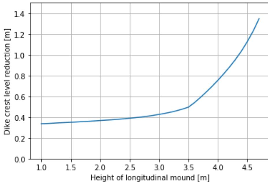
Figure D-20 Dike crest height reduction based on crest height of longitudinal mound for location Waal\_09
