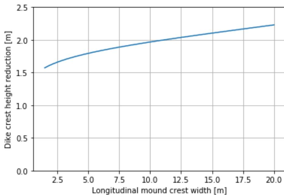
Figure D-7 Dike crest height reduction based on crest width of longitudinal mound for location Lek\_05
