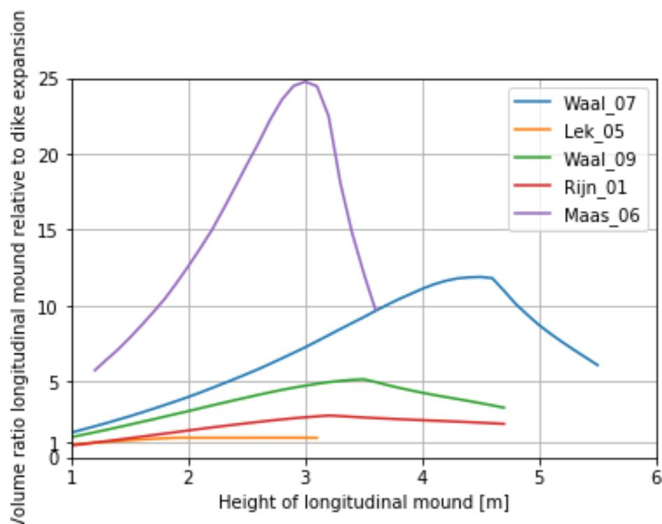
Figure D-34 Volume ratio based on crest height of longitudinal mound for all locations
