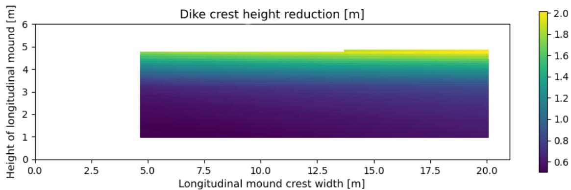
Figure D-15 Dike crest height in metres for all combination of width and length of the longitudinal mound for location Rijn\_01
