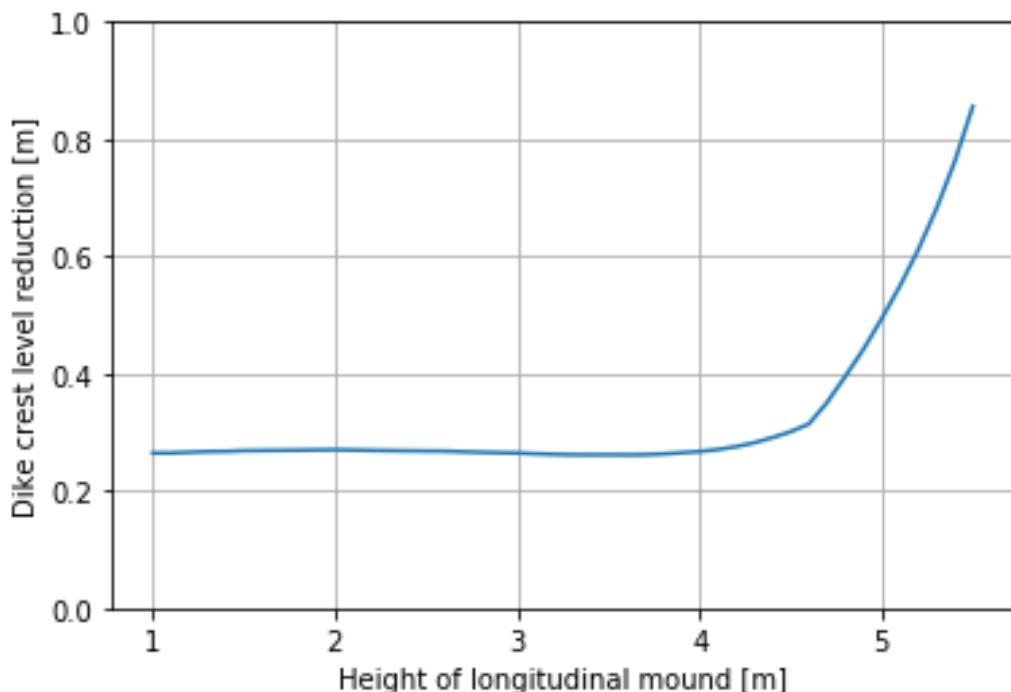
Figure 35 Dike crest height reduction based on crest height of longitudinal mound
