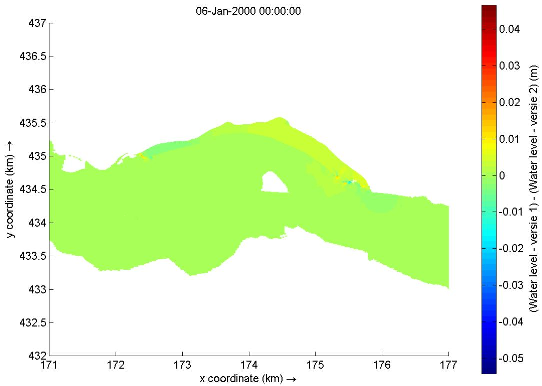
Figure F-4 Water level differences between variant 1 and variant 2. Red indicates a higher water level and dark blue a lower water level for variant 1 than variant 2
