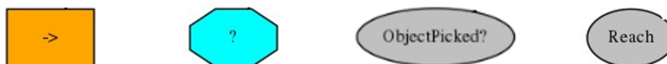
Figure 1: (From Left to Right) Sequence : Succeeds if all children N succeed. Fallback : Succeeds if one child M of N children succeeds. Condition : Checks if a certain condition or world state has been achieved. Leaf : or action node, represents an executable file or (partial) behaviour/skill.
