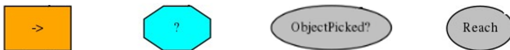
Figure 3.8: (From Left to Right) Sequence : Succeeds if all children N succeed. Fallback : Succeeds if one child M of N children succeeds. Condition : Checks if a certain condition or world state has been achieved. Leaf : or action node, represents an executable file or robot skill.
