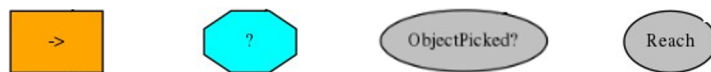
Figure 2: (From Left to Right) Sequence : Succeeds if all children N succeed. Fallback : Succeeds if one child M of N children succeeds. Condition : Checks if a certain condition or world state has been achieved. Leaf : or action node, represents an executable file or (partial) behaviour/skill.
