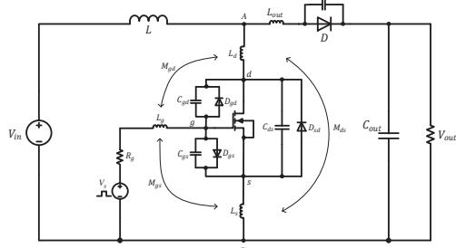
Fig.1 GaN GIT based boost converter with circuit and package parasitics
