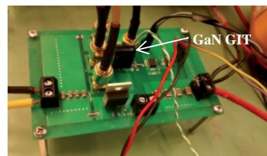
Fig.5 Converter prototype employing GaN GIT
