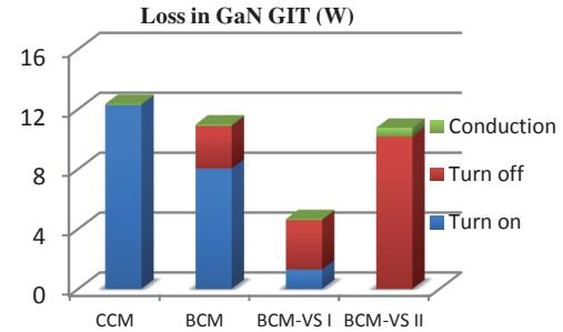
Fig. 3 Loss breakdown of GIT in different modes
