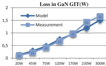
Fig. 6 Measured and calculated (modeled) loss in GaN GIT
