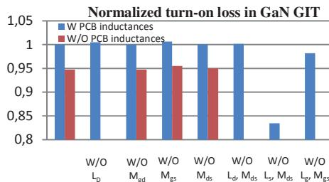
Fig.4 Effects of parasitic inductances in CCM on turn-on loss
