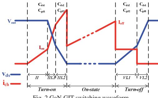
Fig. 2 GaN GIT switching waveform
