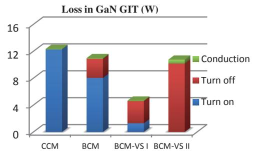
Fig. 3 Loss breakdown of GIT in different modes
