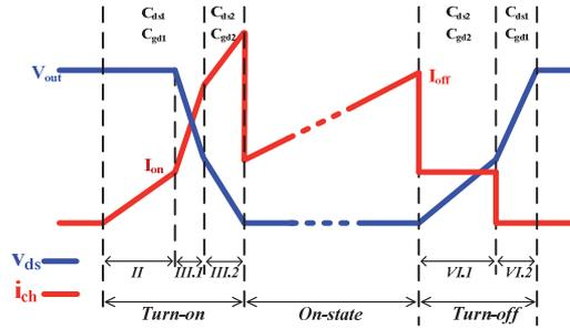
Fig. 2 GaN GIT switching waveform
