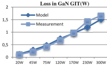
Fig. 6 Measured and calculated (modeled) loss in GaN GIT
