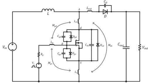
Fig.1 GaN GIT based boost converter with circuit and package parasitics
