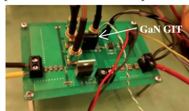
Fig.5 Converter prototype employing GaN GIT
