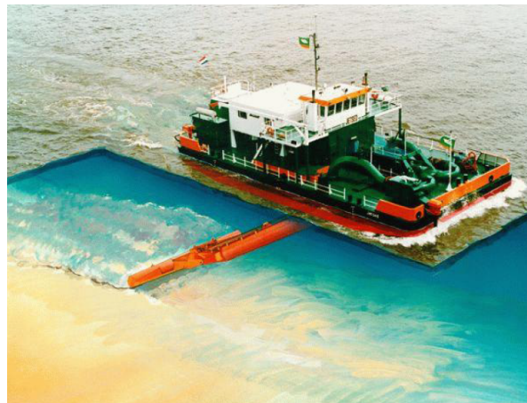
Figure H.5: Water injection dredging (Verhagen, 2000).
