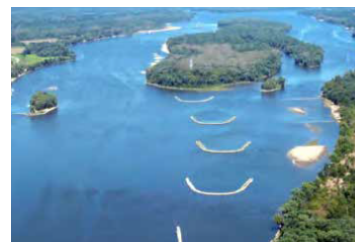
(c) Series of chevron dikes in the Mississippi river (United States Army Corps of Engineers, 2012).
