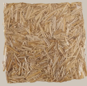
Starch binder 8 g starch · 80 ml Water
