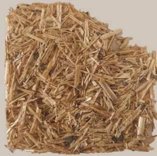
Tannin binder 8 g starch · 16 ml Water · 0.7 g lime
