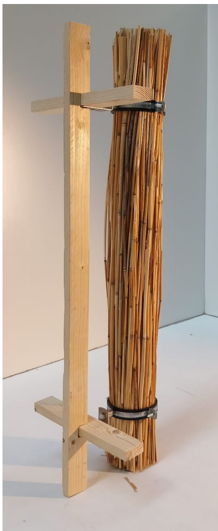
Fig. 35: Physical model to explore arch-roof connections
