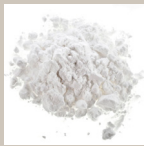
Starch binder 8 g starch · 80 ml Water
