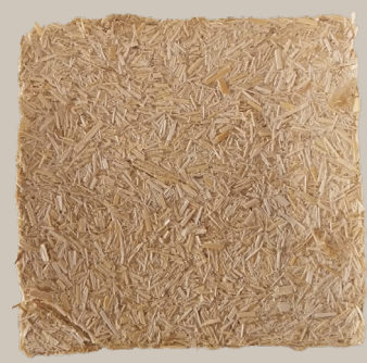
Starch binder 8 g starch · 80 ml Water
