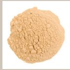
Tannin binder 8 g starch · 16 ml Water · 0.7 g lime
