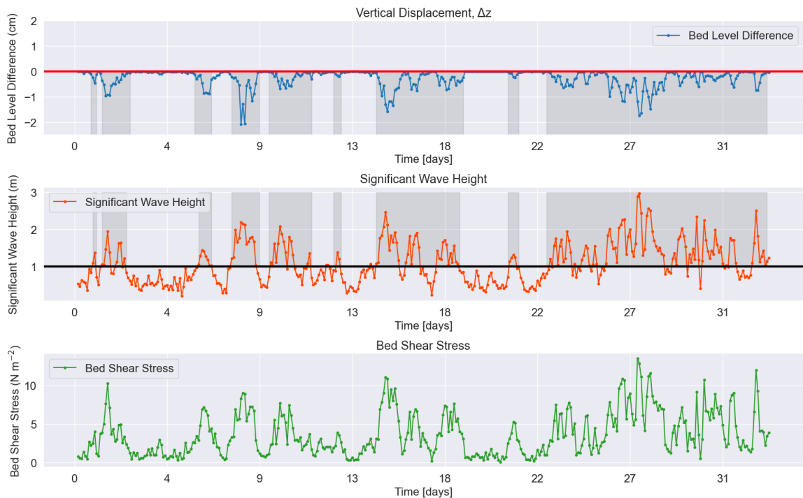
Figure 41: Artificial flattening of nourishment crest as modeled with the standard model. Vertical displacement of the nourishment crest, \Delta z , is primarily driven by wave height, revealing faster flattening with increasing wave heights. Minimal flattening is observed for wave heights below 1.0m, while significant displacement occurs for waves exceeding 1m in height. A gradual reduction in magnitude over time suggests approaching equilibrium. Although tide-induced flow variation may influence erosion slightly, model results indicate wave height predominantly governs flattening.
