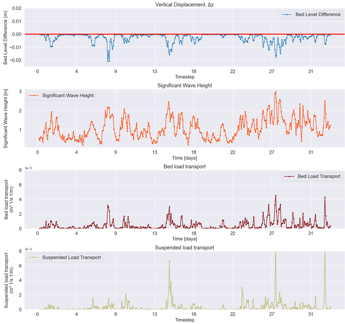
Figure 43: Comparison of bed load and suspended load transport contributions in sediment transport, aiming to identify the dominant mechanism driving the flattening of the nourishment. While bed load transport appears slightly more pronounced overall, three distinct peaks in suspended load transport suggest instances where it significantly exceeds bed load transport.
