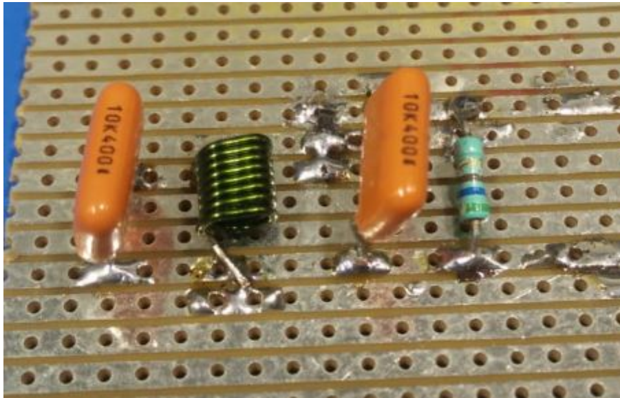
Figure 4.27: Final detector circuit
