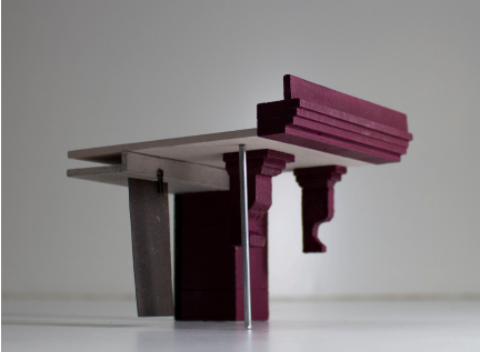
Own work: Joint model, 1:20, Key: brown - function, purple - ornamentation, shell - silent, texture - appropriated areas
