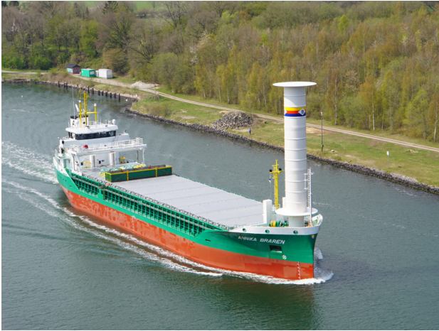
Figure 5: M/V Annika Braren equipped with "Eco Flettner 1" type rotors (Eco-Flettner, nd).
