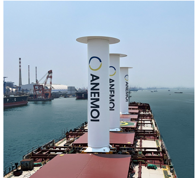
Figure 2: TR Lady equipped with "Anemoi 4" type rotors (Anemoi, nd).
