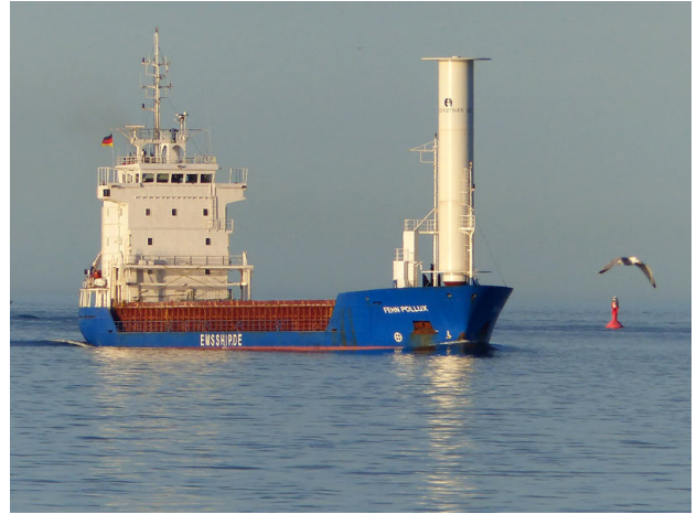
Figure 6: M/V Fehn Pollux equipped with "Eco Flettner 1" type rotors (Eco-Flettner, nd).
