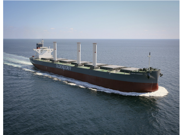
Figure 4: Dietrich Oldendorff equipped with "Norsepower 3" type rotors (Norsepower, nd).
