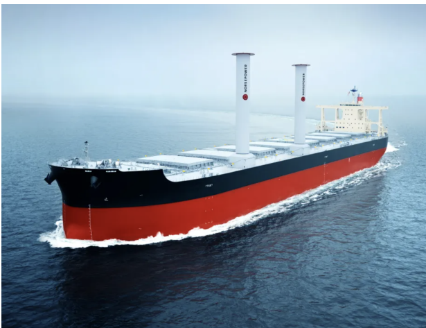
Figure 3: Camellia Dream equipped with "Norsepower 6" type rotors (Norsepower, nd).
