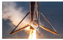
(b) Telescopic landing legs with secondary Y-strut 7
