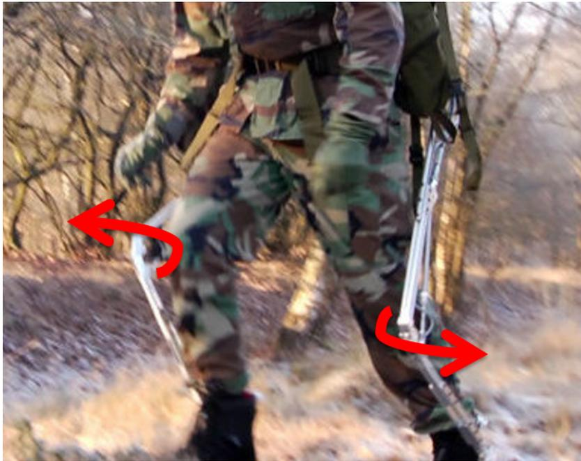
Figure 1.2: The legs of the Exobuddy tend to rotate outward during operation, increasing the risk of collision with obstacles.
