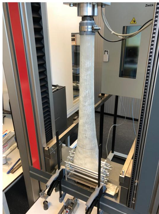
Figure 4.8: Test setup for Experiment 2, here the drum is constrained and can not rotate. The top connection is spherical, whereas the bottom connection is fixed.
