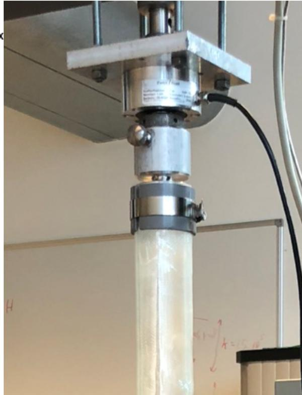
Figure 4.5: End conditions of the STEM for Experiment 1: the end of the STEM is constrained into a tubular shape and connected to the tensile tester through a spherical joint.
