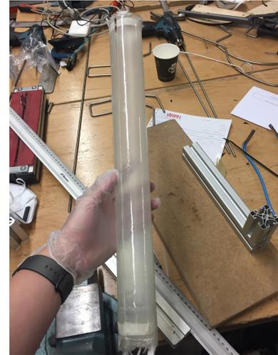
(c): The STEM after curing and removing from the mould. The ends remain to be cut.
