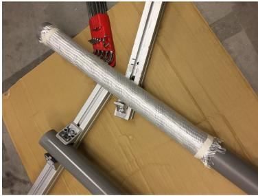
(a): The glass fibre sleeve is fixed onto the PVC mould
