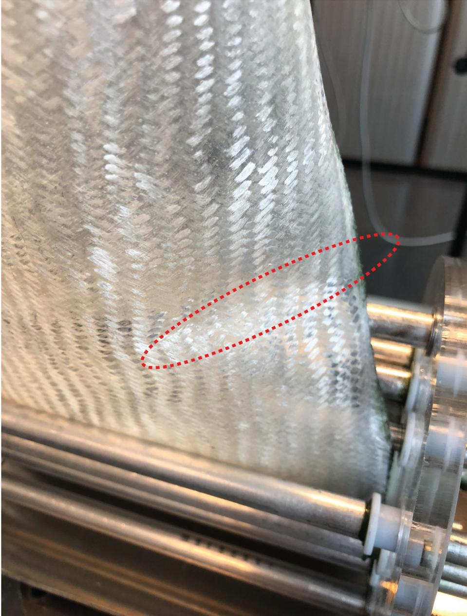
Figure 4.10: Failure during STEM compression takes form as a dent propagating in the material, after which the STEM continues to crumple and lose its load-bearing capacity.
