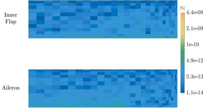
(a) Aerodynamic sensitivity errors: inboard and outboard control-surface deflections.
