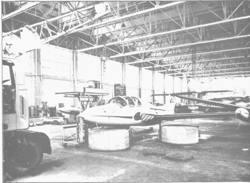
FIG. 3. DETERMINATION OF THE AIRCRAFT CENTRE OF GRAVITY
