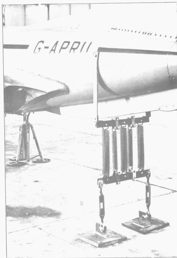
FIG. 6. SHOWING METHOD OF SPRING ATTACHMENT USED IN PITCHING RIG
