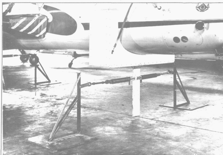
FIG. 10. DETAIL OF CRADLE AND SPRING ATTACHMENT SYSTEM USED IN THE YAWING RIG
