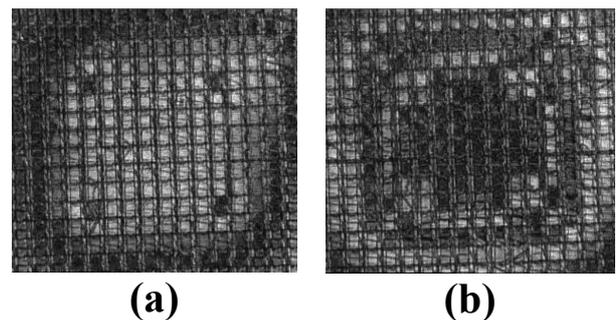
Fig. 8. Combined influence of four active pixels; frequency of the square waves 1 kHz, amplitude  $V_1$  for 4 adjacent active pixels in the center and  $V_2 = 4.5$  V for other ones. Values of  $V_1$ : 3.5 V (a) and 2.5 V (b).
