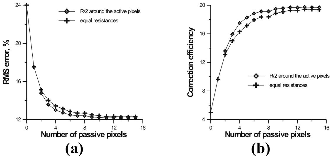
Fig. 2. *Rms* correction error (a) and correction efficiency (b) of 36-channel LC-MWC based on discrete IC resistors vs number of passive pixels placed between two adjacent active pixels.
