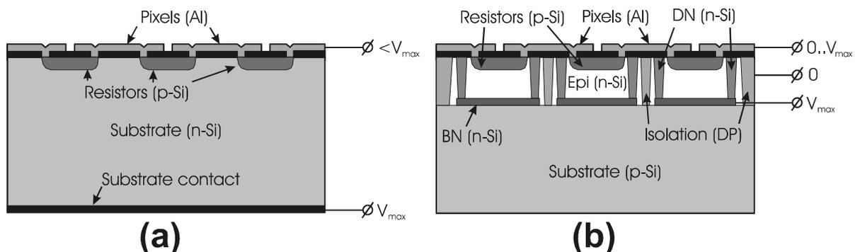
Fig. 4. Implementation of diffusion resistors in a custom (a) and a bipolar (b) processes.
