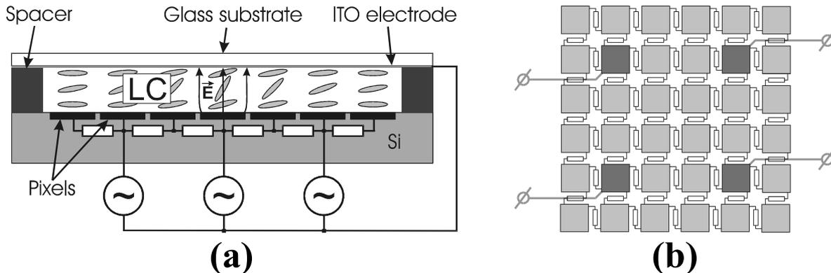
Fig. 1. Cross-section (a) and structure of pixels (b) of the hybrid LC wavefront corrector.
