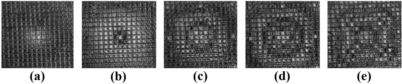
Fig. 7. Visualization of the influence function of an active pixel; frequency of the square waves 1 kHz, amplitude  $V_1 = 4.5$  V for the active pixel in the center and  $V_2$  for other active pixels. Values of  $V_2$  are 4 V (a), 3.5 V (b), 3 V (c), 2.75 V (d) and 2.25 V (e).
