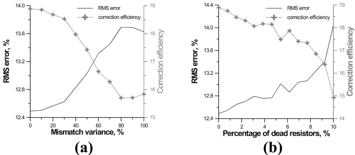
Fig. 3. *Rms* correction error and correction efficiency of 36-channel LC-MWC vs resistors' mismatch variance (a) and percentage of "dead" (open-circuit) resistors (b).
