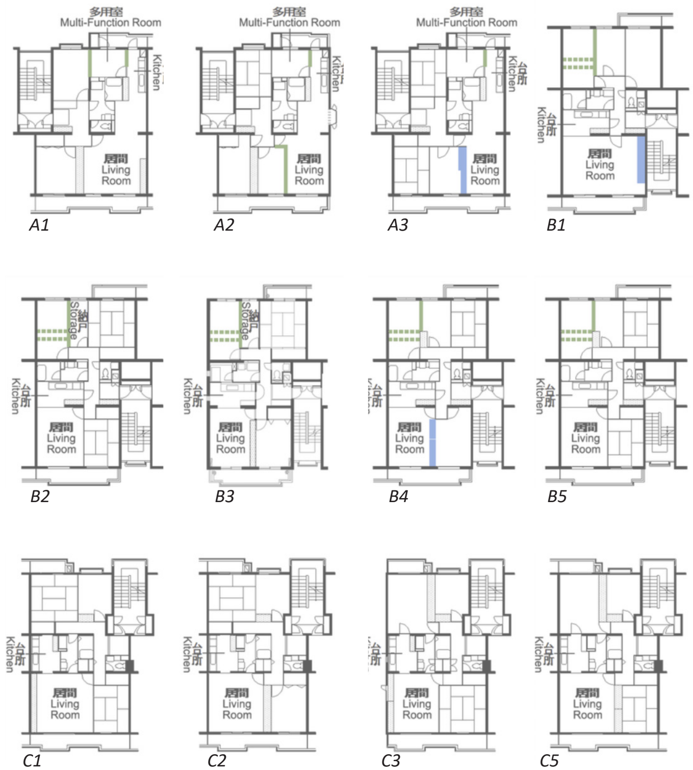
Figure 36 Plan types in Tsurumaki 3, for a four-story apartment. The top of the drawing indicates north. Blue: Relocatable storage unit; Green: Movable partition wall.
