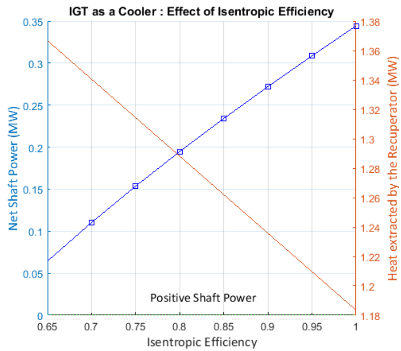
Figure E.4: Simulation results of producing work and heat from an IBC system cooling flue gas stream from the combustor of the gasifier system
