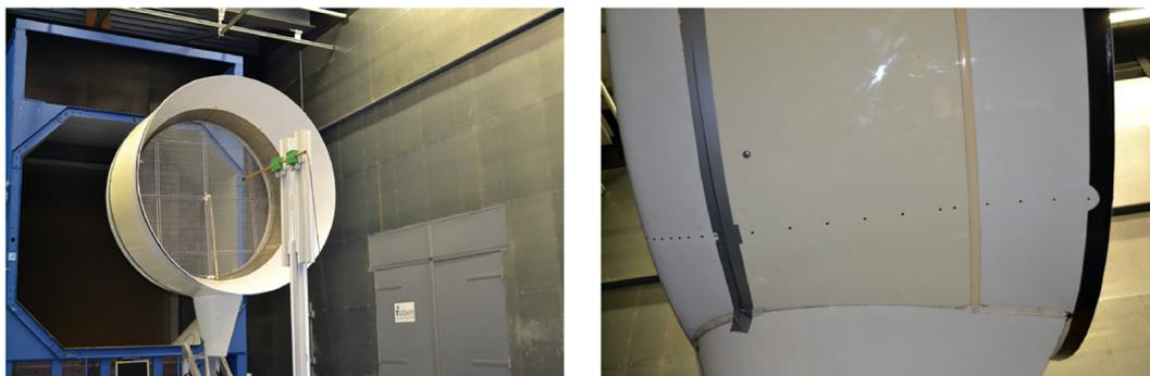
**FIGURE 2** Pictures showing the experimental set-up with hot-wire anemometer placed on the traversing system (left) and pressure taps along the duct surface (right) [Colour figure can be viewed at [wileyonlinelibrary.com](http://wileyonlinelibrary.com)]
