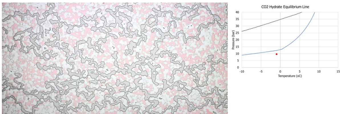
Figure 4.19: Micromodel image at 9.75 bars and -1^\circ\text{C} during the dissociation process, showing hydrate dissociation when pressure and temperature conditions are outside the hydrate stability zone.
