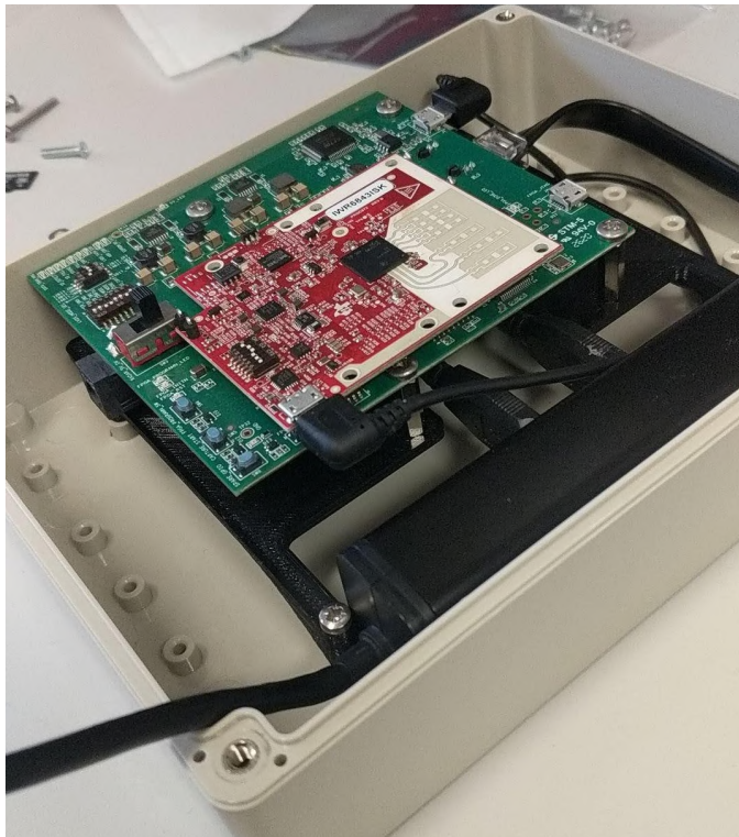
Figure 5.5: Supporting board with the radar in the plastic container, used for the data collection on neonates performed by C. Ramsey at Erasmus Medical Center [8]
