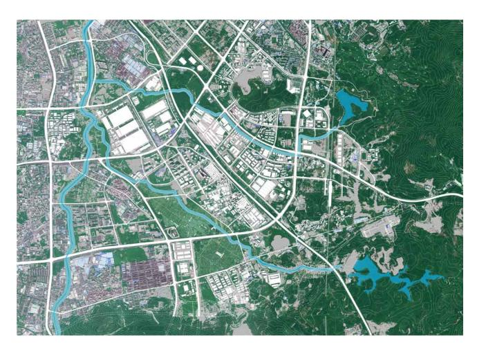
Fig 159 Landcover's permeability in the pilot area: green- permeable; white- buildings and infrastructure; grey- exposed soil
