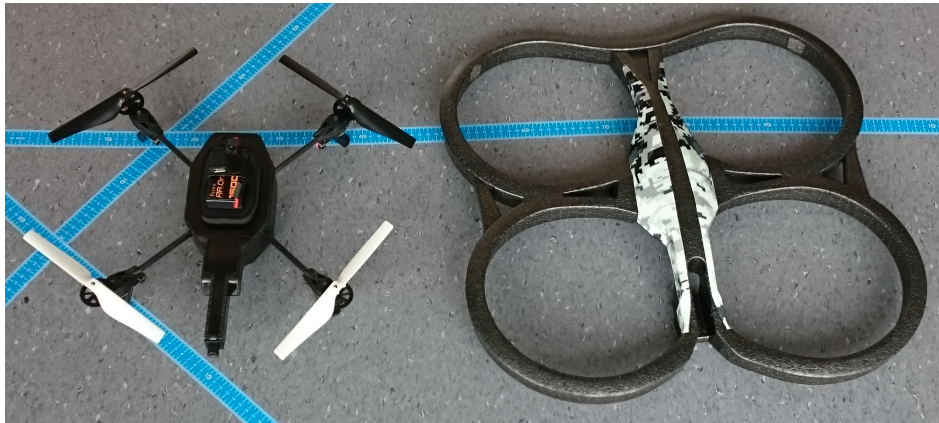
Figure 4-3: Parrot AR.Drone 2.0 with Parrot battery attached and indoor hull detached.
