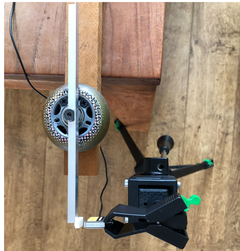
Figure B-13: Setup to determine friction of ball bearing.
