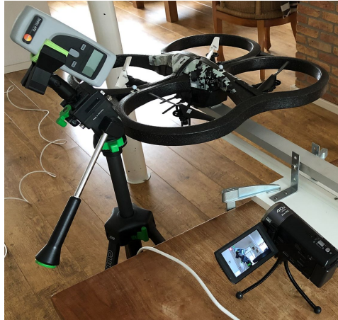
Figure B-9: Digital hand-tachometer mounted on tripod with a camera pointing to the tachometer.
