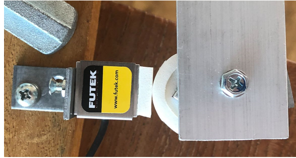
Figure B-12: Sensor contact point in torque setup.
