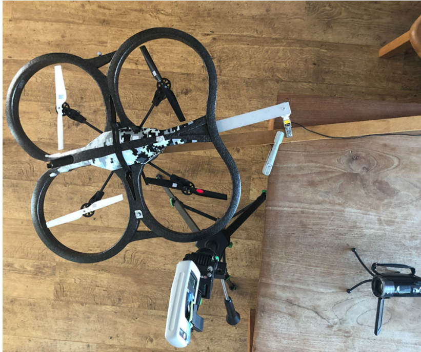
Figure 5-11: Setup to determine torque coefficient c_Q .
