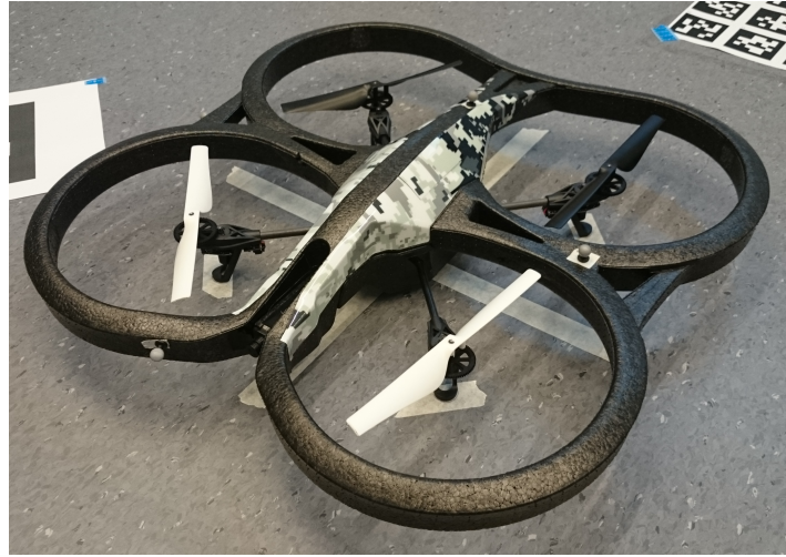
Figure 4-4: Parrot AR.Drone 2.0 with indoor hull and OptiTrack markers attached.
