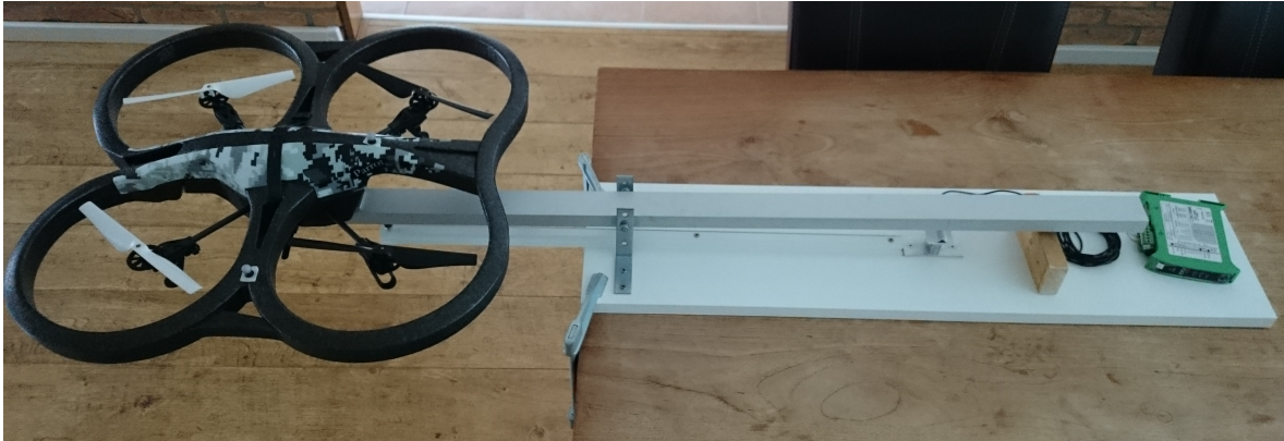
Figure 5-8: Setup to determine thrust coefficient c_T .
