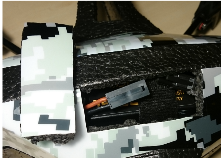
Figure C-3: Replaceable part of indoor hull to be able to power on the quadrotor when aligned with OptiTrack coordinate axes.
