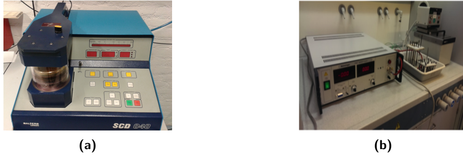
Figure 2.6: Particulate composite preparation pictures: the Balzers Union SCD40 Sputter-coater (a), the poling set-up: DC generator (left), poling jig (central), and silicon oil bath (right) (b).
