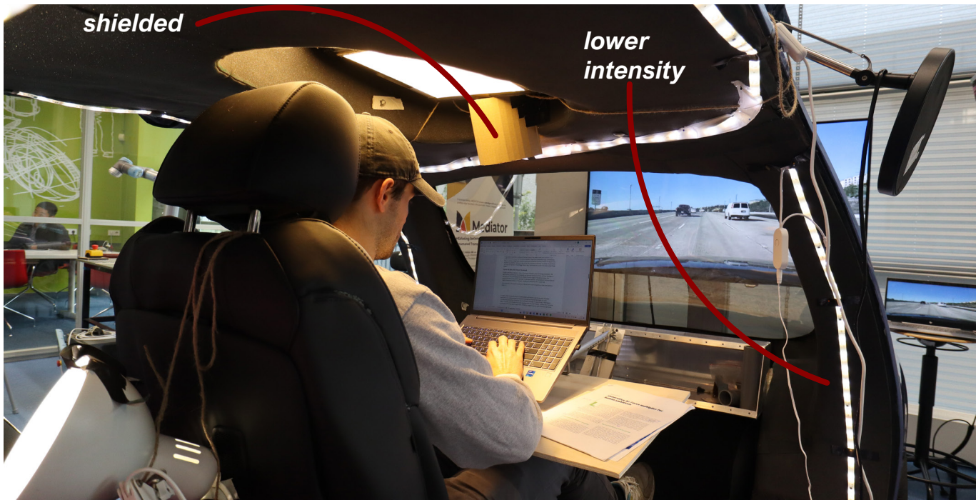
Figure 33: after initial testing the focus light is shielded and the door lights are dimmed JLR | TU Delft
