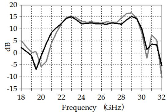
Fig. 3. Directivity of the simulated leaky wave antenna with the FSS designed for identical permittivity  $\epsilon_{r1,2} = 6$  (black line) and for two permittivities  $\epsilon_{r1} = 6$ ,  $\epsilon_{r2} = 10$  (grey line).
