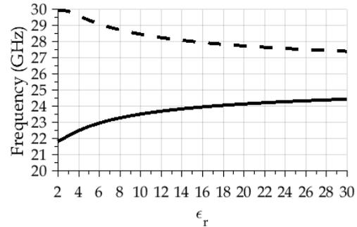
Fig. 1. (a) Frequency variation as a function of the dielectric permittivity for the common solutions of (2), for the inductive (solid line) and capacitive equivalences (dashed line) for  $h_0 = 5.79$  mm.
