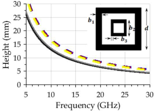
Fig. 2. Solutions for the cavity height as a function of the frequency, for different values of permittivity ( $\epsilon_r = 4, 6, 8, 10, 12$ ) for the inductive (solid lines) and the capacitive (dashed lines). The FSS unit cell is also presented.
