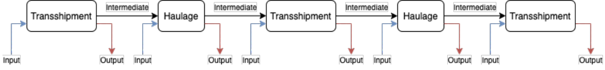
Figure 4.2: Example of IFT-chain with three transshipment and two haulage segments. Besides inputs and outputs for each division, there are intermediates between consecutive divisions.
