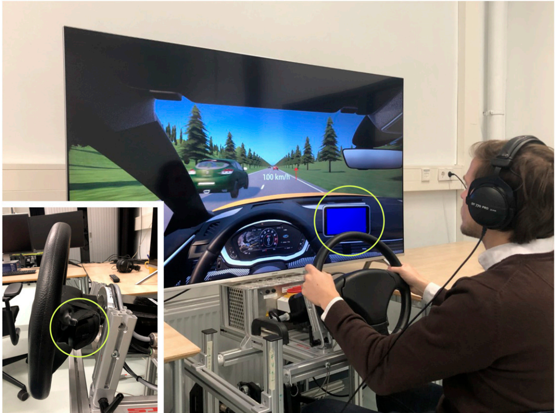
Figure 1. A participant driving in the driving simulator. The dashboard display shows the steering gain (SG) currently active (here colored blue, indicating low SG). The arrow next to the depicted speed indicates the advised SG level (available in the DI condition only). In this figure, participants are advised to switch “up,” from low SG to high SG. The left-bottom inset shows the button on the back of the steering wheel that was used to initiate the SG transitions. Participants wore headphones that displayed regular driving sounds “(Melman, Visser et al., 2021)”.
