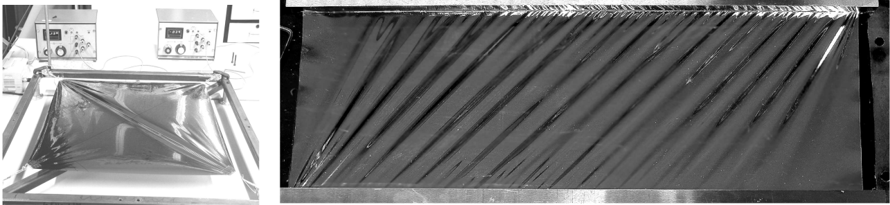
(a) Thin sheet subject to tensional corner loads. The force pair top left and bottom right has 4 times the magnitude of the force pair bottom left and top right.
