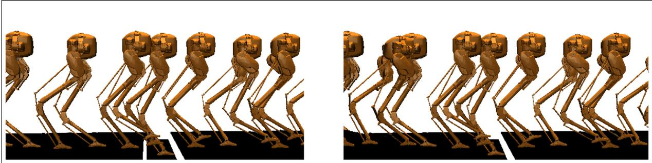
Fig. 9. Gait tiles (associated with the plots in Fig. 8) of Cassie walking down an expected downstep (left) and an unexpected downstep (right).
