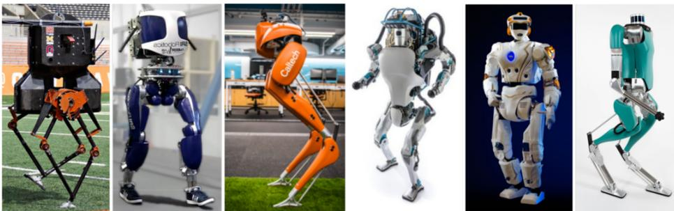
Figure 2.3: Examples of *modern* bipedal robots (from left to right): ATRIAS [34], DURUS [44], Cassie [36], Atlas [51], Valkyrie [56], and Digit [36]. ATRIAS, DURUS, Cassie, and Digit all have structural compliance in their designs.
