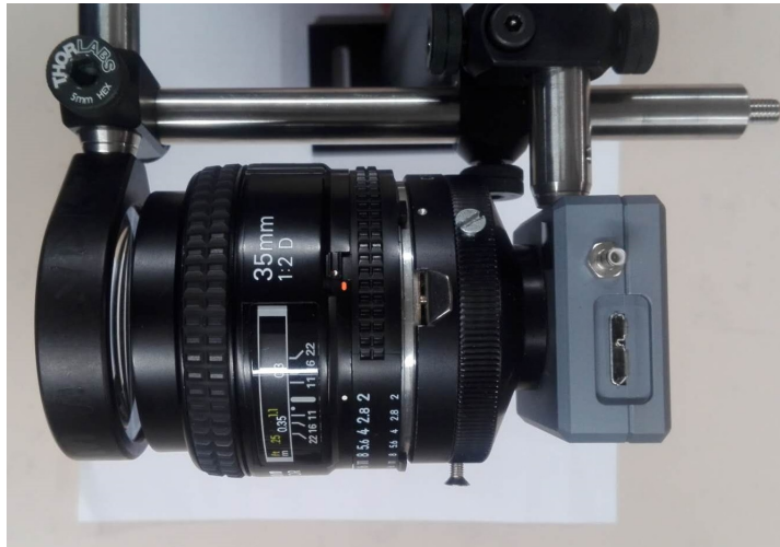
Figure 5.6: The combined camera head which is composed of 3 elements. From left to right: 300mm plano-convex lens, the camera lens, and the imaging sensor.
