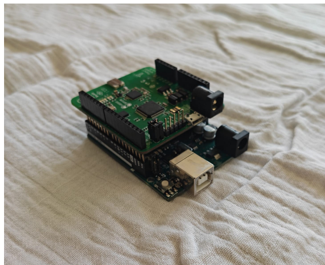
Figure 4.1: The wearable; including the developer tag (top) and the Arduino Uno (bottom)
