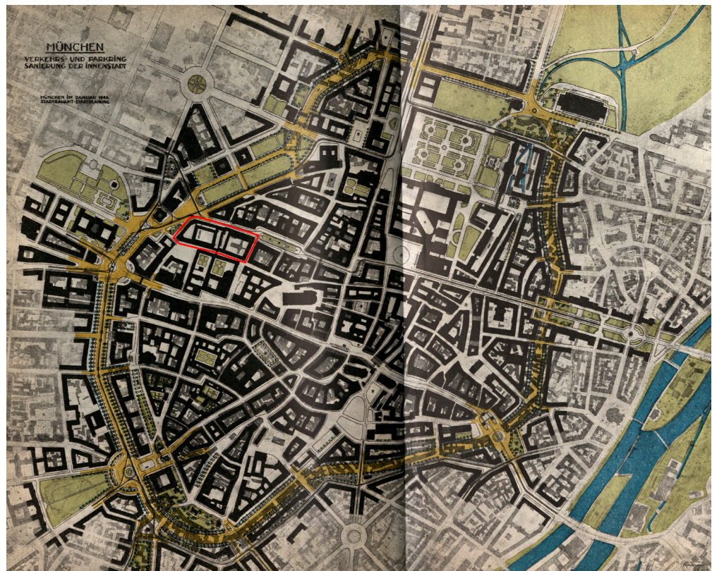
Figure 18: Plan for the reconstruction of Munich's city centre by Karl Meitinger (light grey: old building structures, black: new proposal)
