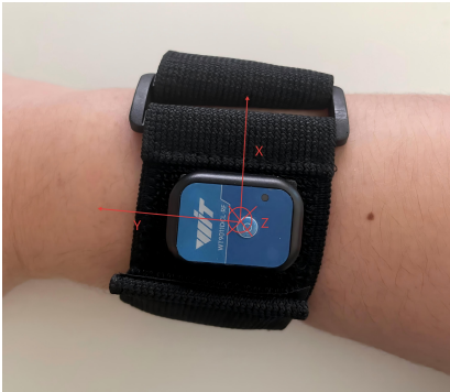
Fig. 8: Position and Orientation of IMU Sensor
