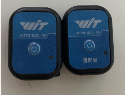
Fig. 7: IMU Sensor(left) and its Adapter(right)
