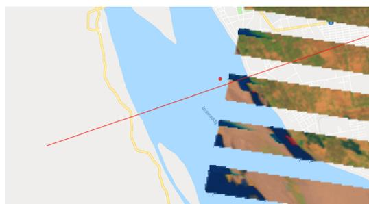
Figure 2.10: Cross-section at the Magway station at 23-03-2007. The satellite image only covers part of the cross-section, resulting in a too low estimate of river width.
